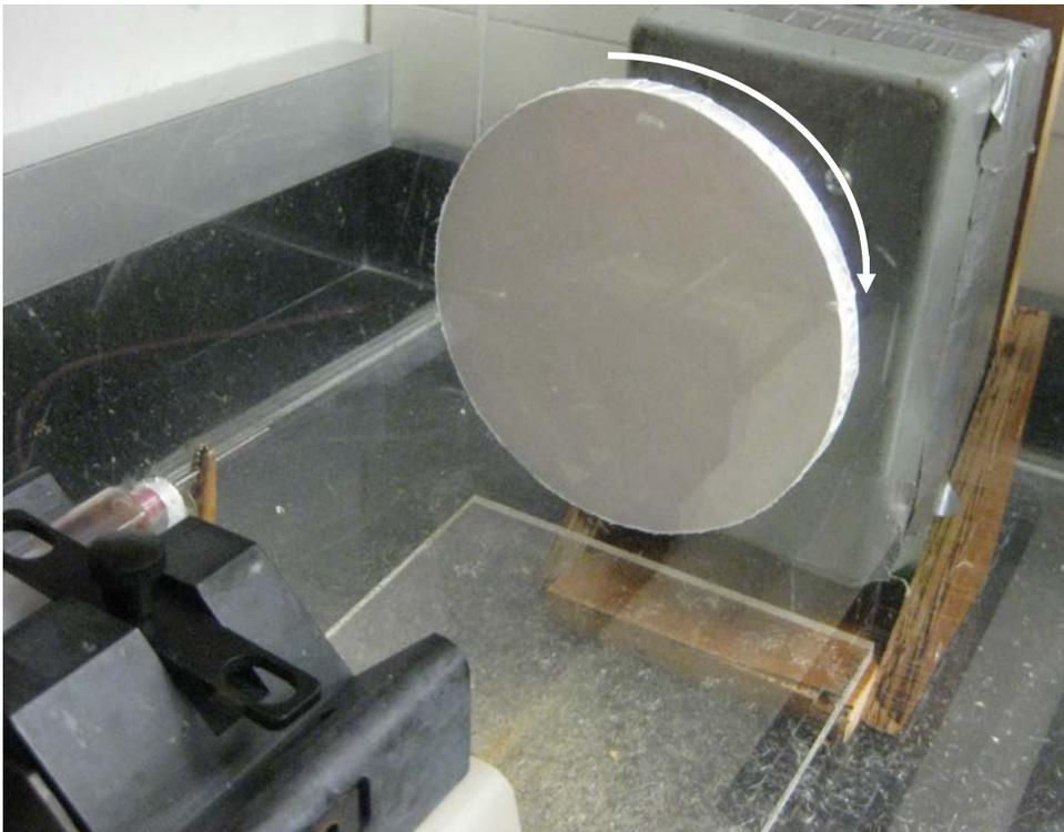
**Figure 1.2 – View of the collection target with nano-fibrous chitosan accumulation.**
