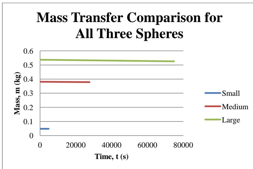
**Figure 8:** Comparison of mass sublimation rates for all three spheres to determine if they are parallel over longest time frame.
