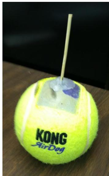
**Figure 1:** Test sample recently sealed within tennis ball mold using a wax cap.
