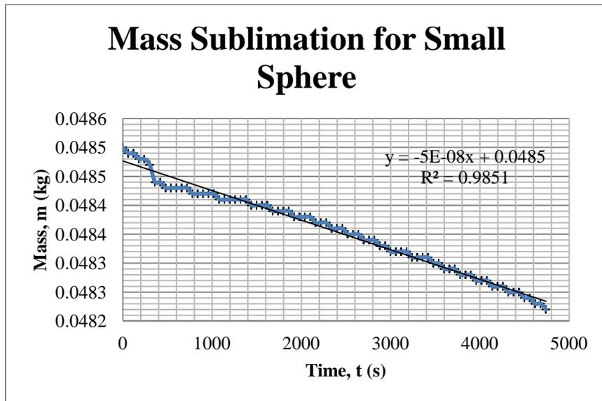
**Figure 5:** Mass loss of small diameter sphere as measured in 60 second intervals.
