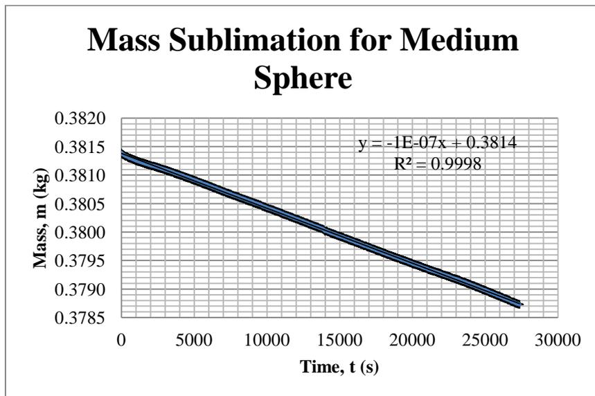
**Figure 6:** Mass loss of medium diameter sphere as measured in 60 second intervals.
