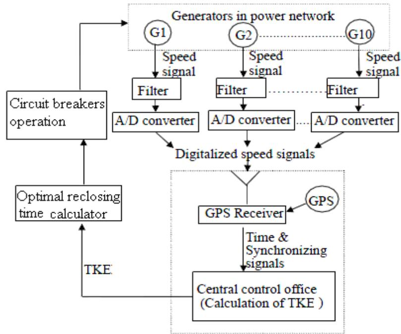
Figure 11: Closed loop circuit breaker control system
