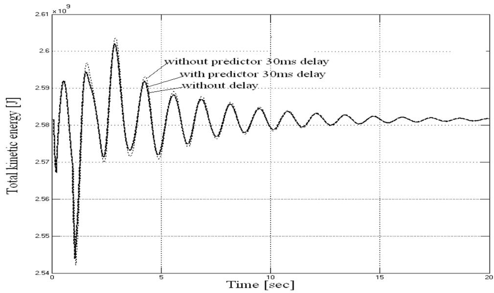
Figure 19: Responses for with and without predictor in case of 3LG permanent fault at F2 in 30ms delayed system
