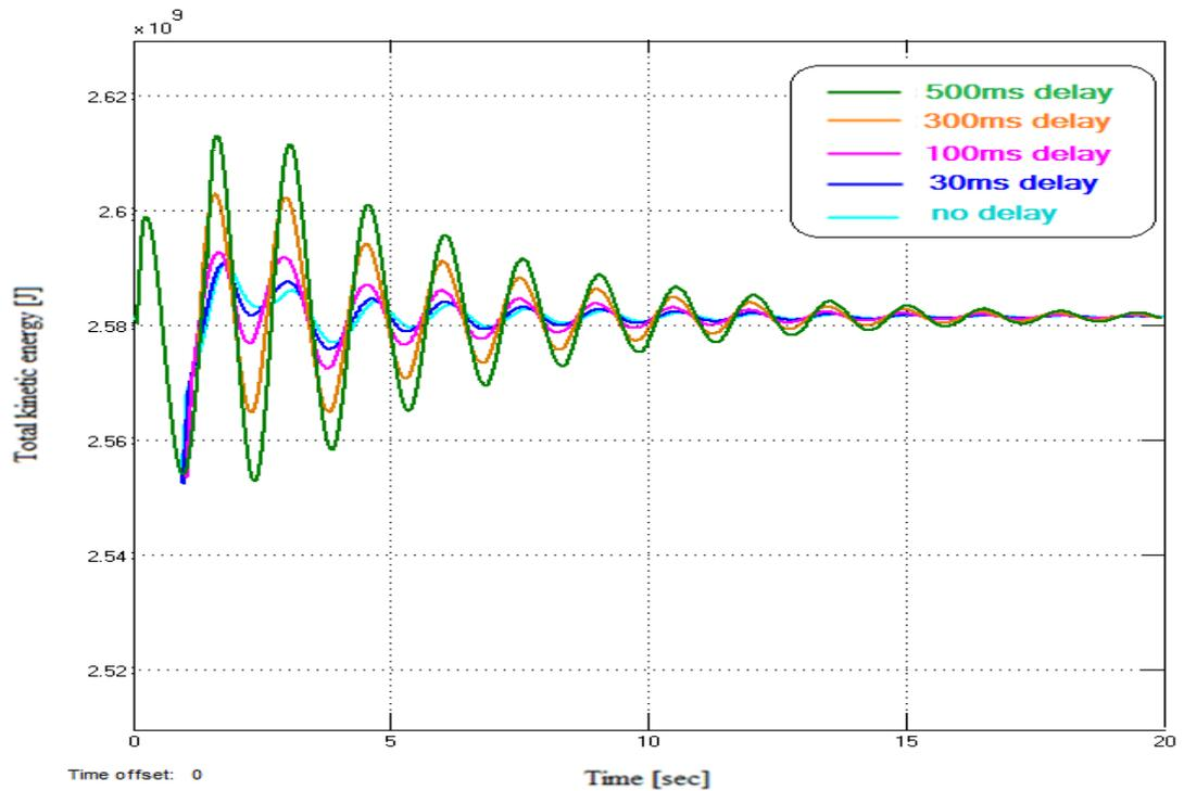
(a)TKE response for 3LG permanent fault at F1
