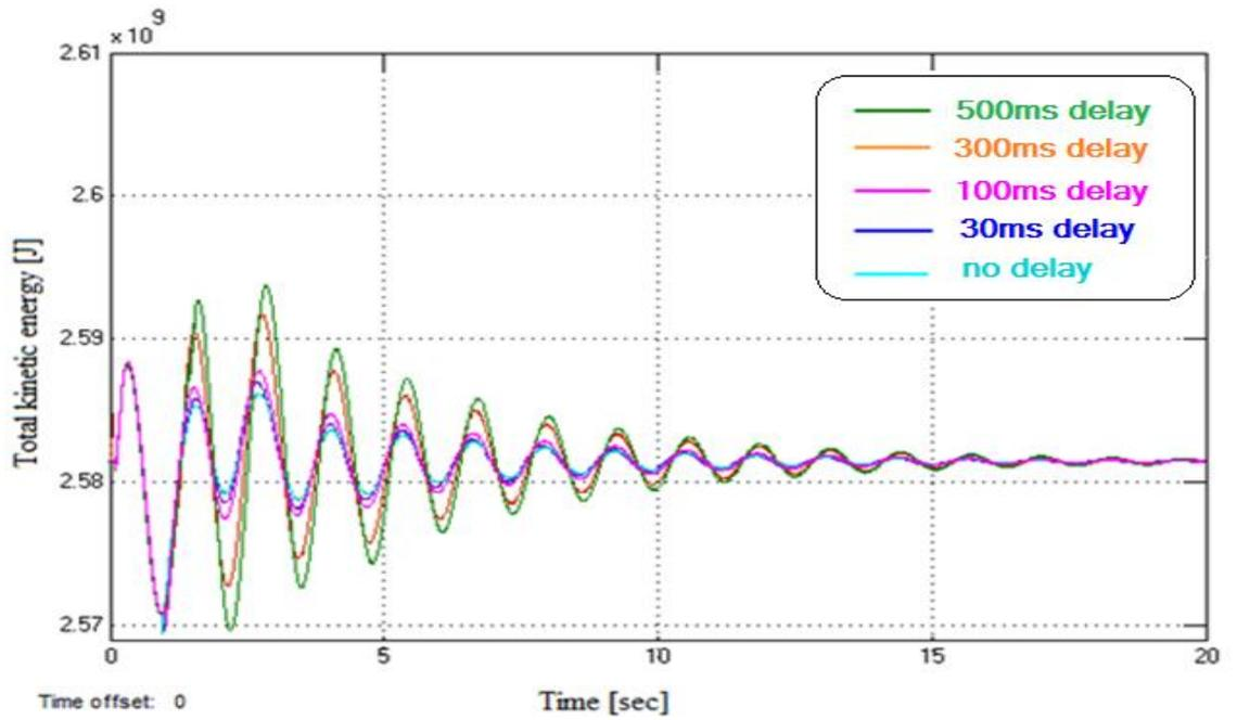
(b) TKE response for 2LL permanent fault at F1
