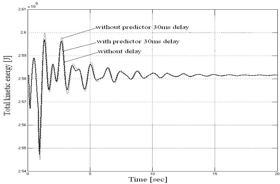
Figure 20: Responses for with and without predictor in case of 3LG permanent fault at F3 in 30ms delay system
