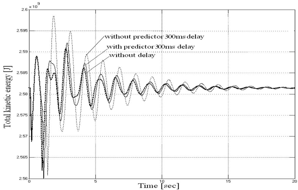
Figure 18: Responses for with and without predictor in case of 1LG permanent fault at F2 in 300ms delayed system
