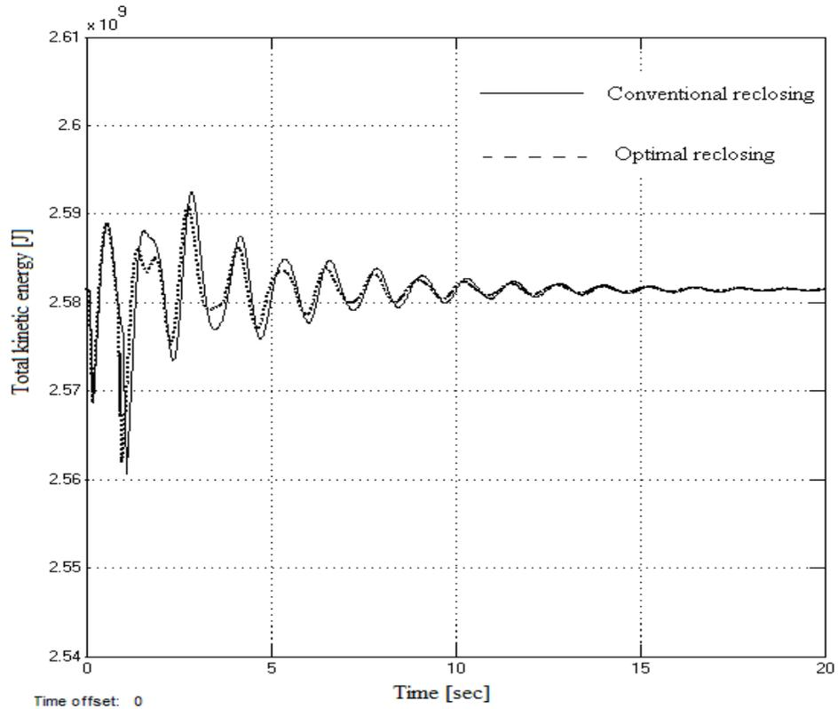
(b) 1LG permanent fault at F2
