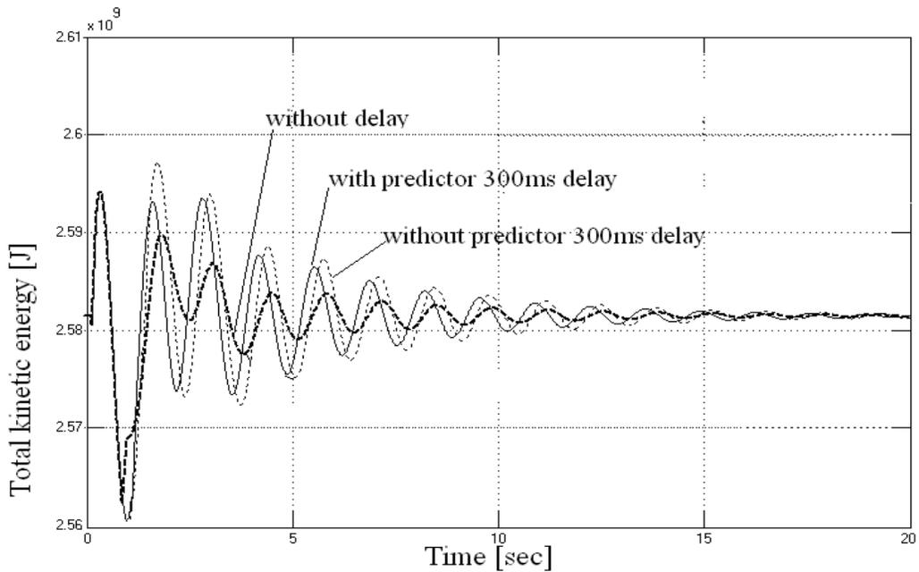
Figure 16: Responses for with and without predictor in case of 3LG permanent fault at F1 in 300ms delayed system
