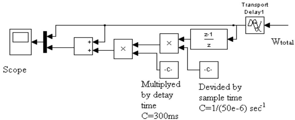
Figure 15: Predicted method simulated in Matlab/Simulink
