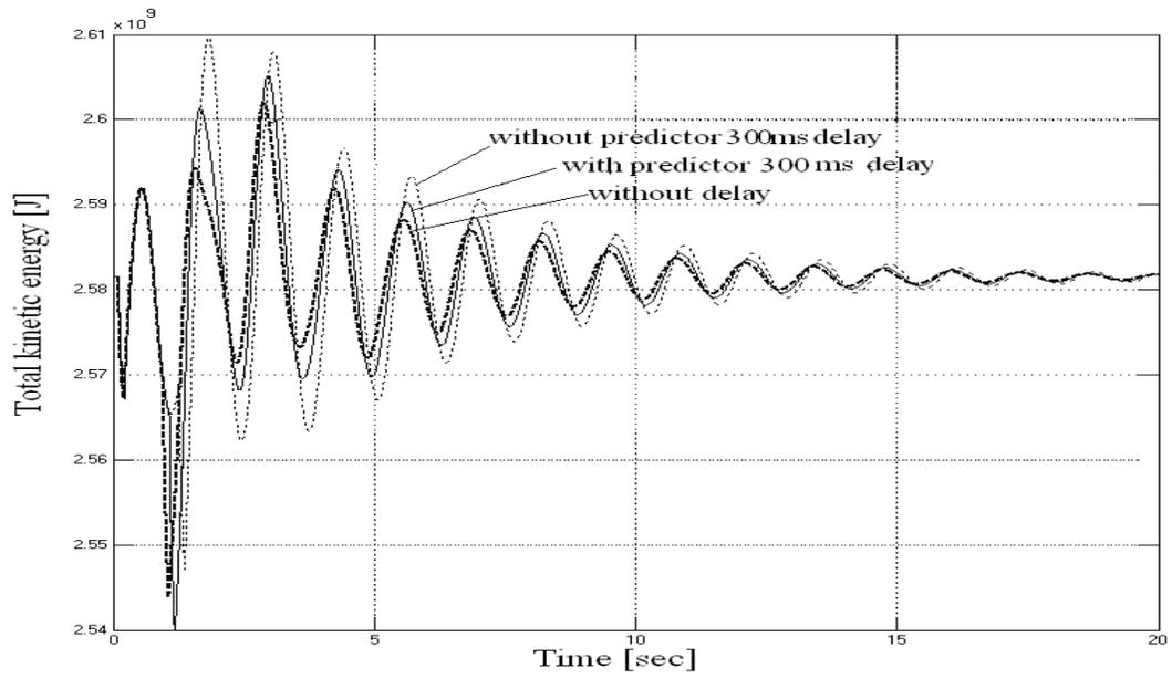
Figure 17: Responses for with and without predictor in case of 3LG permanent fault at F2 in 300ms delayed system
