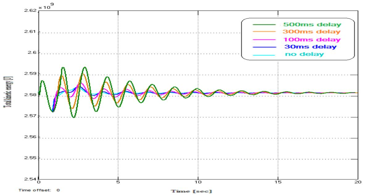
(c) TKE response for 2LL permanent fault at F1
