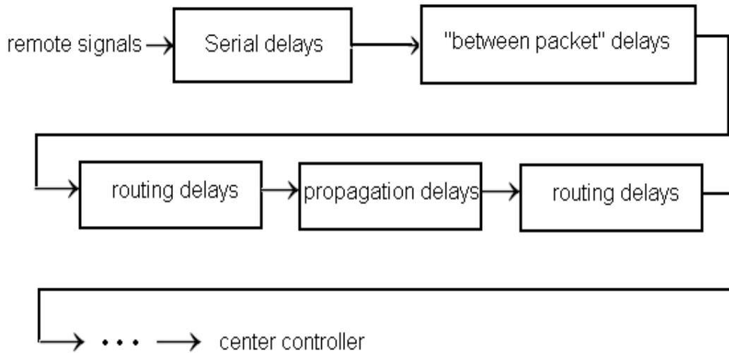
Figure 2: Transmission of Remote Signals
