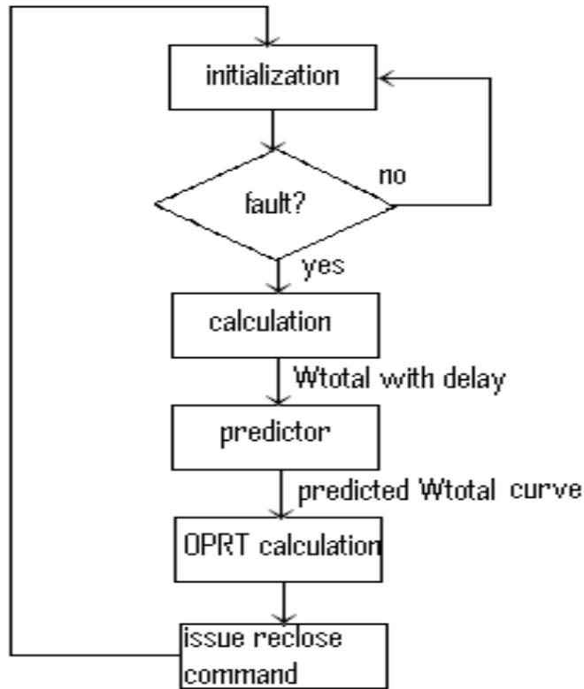
Figure 4: Flow chart diagram of OPTR with predictor
