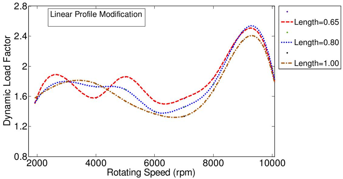
Figure 3.52 Effect of profile modification length on gear dynamic load. Full-sine spacing error with linear profile modification, and maximum cumulative tooth spacing error at 0.0003 in ( $\Delta=100\%$ ).
