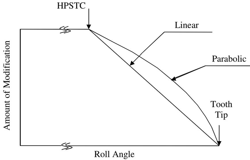
Figure 3.3 Two types of gear tooth profile modification: linear and parabolic.
