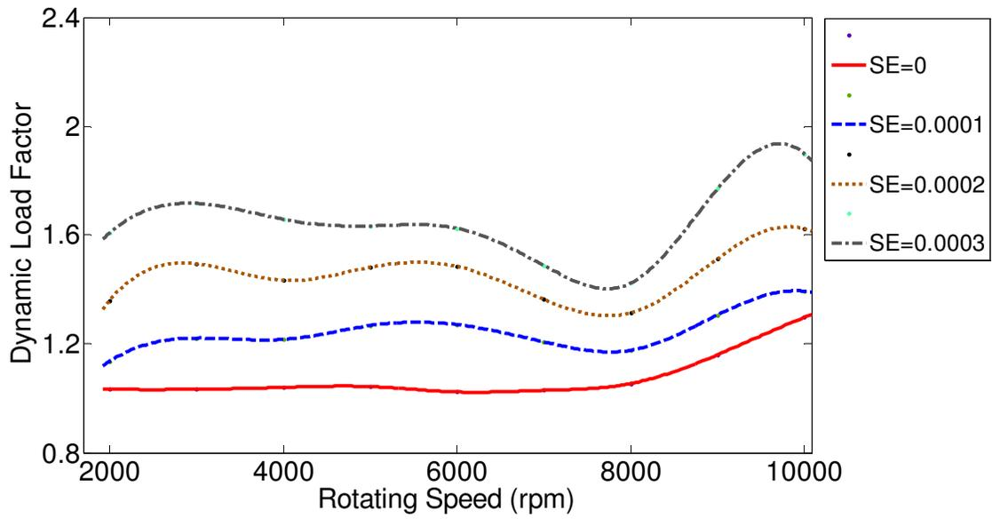
Figure 3.43 Effect of full amount and length of linear tooth profile modification with maximum cumulative random type tooth spacing error from 0 to 0.0003 in.
