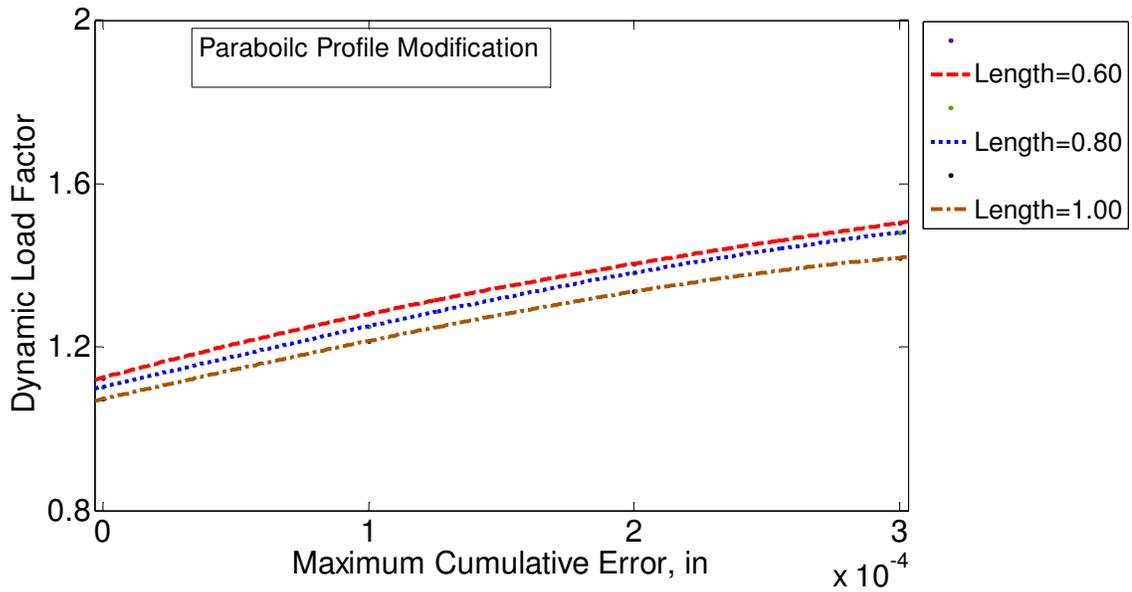
Figure 3.27 Effect of the length of profile modification on half-sine type of spacing error with parabolic modification ( $\Delta=100\%$ ).
