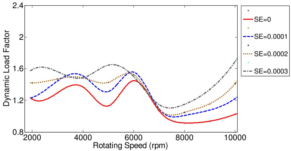
Figure 3.42 Non-modified tooth profile with maximum cumulative half-sine type tooth spacing error from 0 to 0.0003 in.
