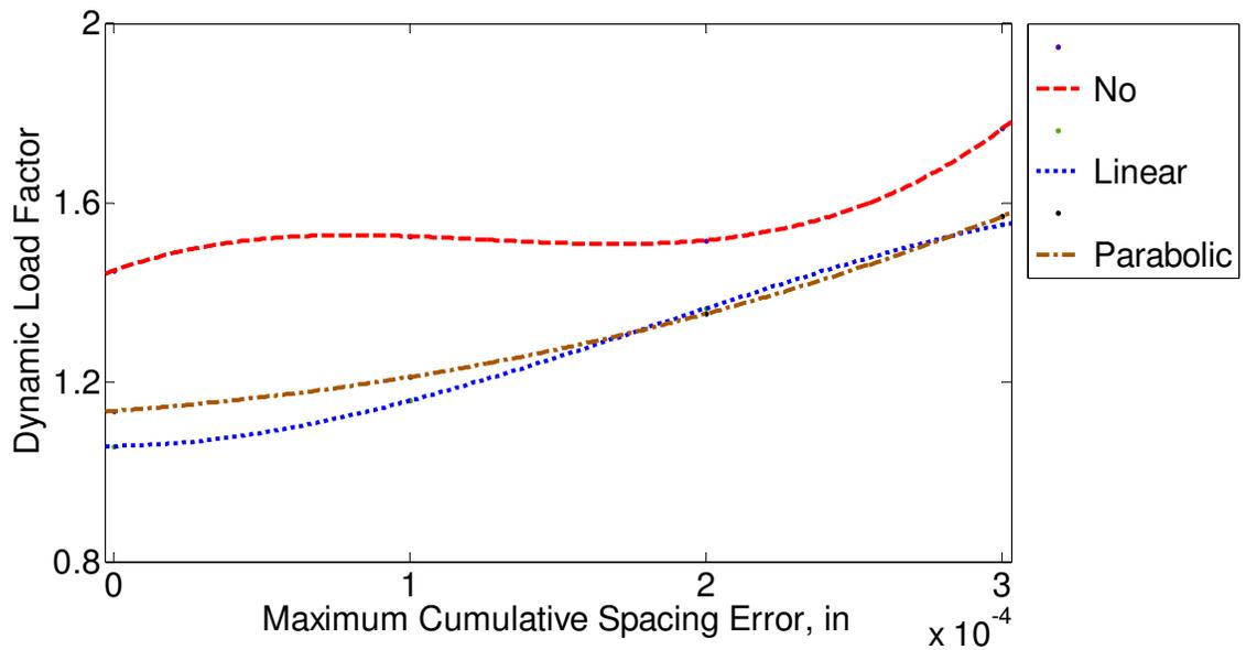
Figure 3.10 Random type of spacing error with no-modification, linear and parabolic modifications ( $\Delta=50\%$ ,  $L_n=100\%$ ).
