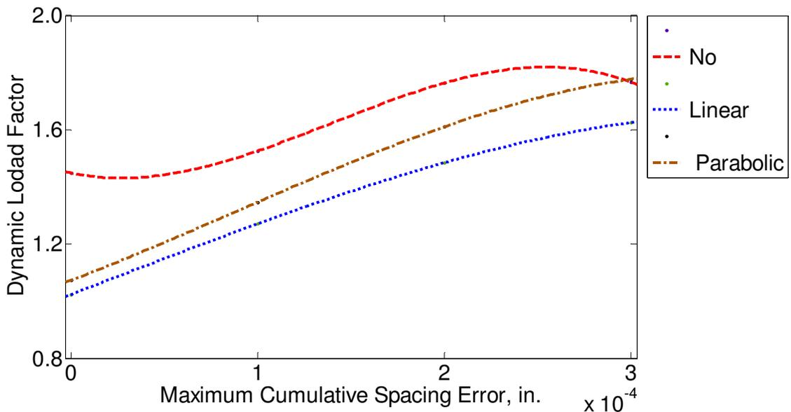
Figure 3.4 Random type of spacing error with no-modification, linear and parabolic modifications ( $\Delta=100\%$ ,  $L_n=100\%$ ).
