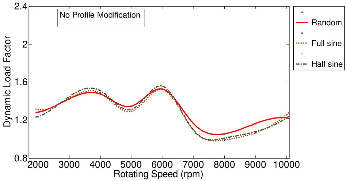
Figure 3.36 Dynamic load factors of sample gears with random, full-sine and half-sine waves of spacing error at 0.0001 in and no profile modification.
