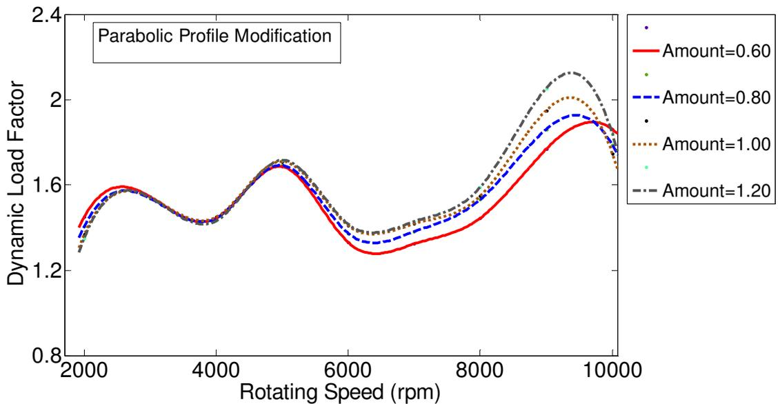
Figure 3.71 Effect of profile modification amount on gear dynamics, for parabolic tooth profile modification with maximum cumulative full-sine type tooth spacing error of 0.0002 in. The modification amount varies from 0.60 to 1.20, and the length is 100%.
