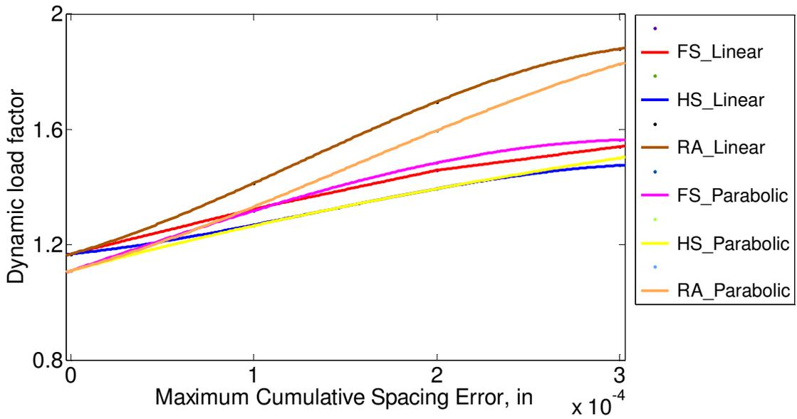
Figure 3.14 Comparison of different type tooth spacing error and profile modifications for ( $\Delta=100\%$ ,  $L_n=65\%$ ).
