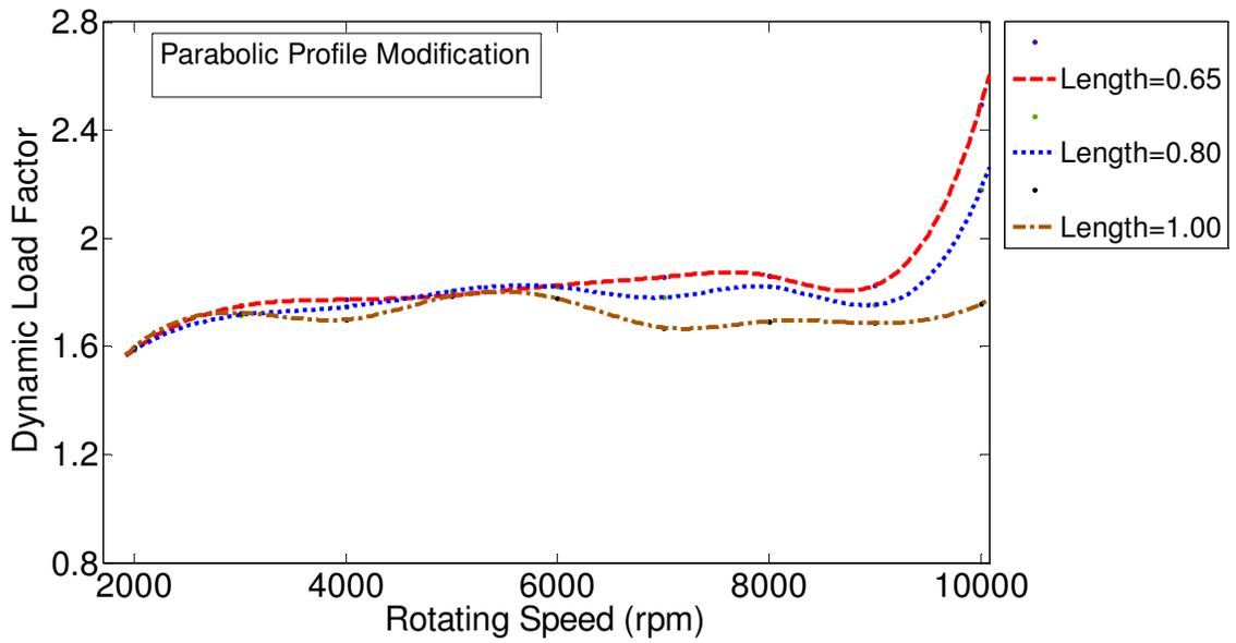
Figure 3.56 Effect of profile modification length on gear dynamic load. Random spacing error with parabolic profile modification, and maximum cumulative tooth spacing error at 0.0003 in ( $\Delta=100\%$ ).
