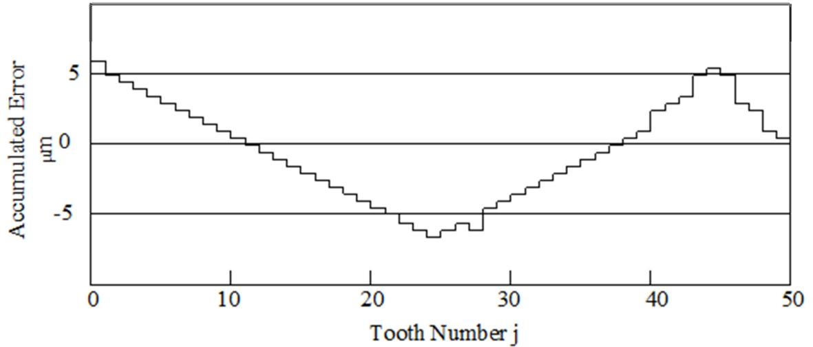
Figure 2.5 Typical Tooth Spacing Errors of a Gear (pitch error graph)
