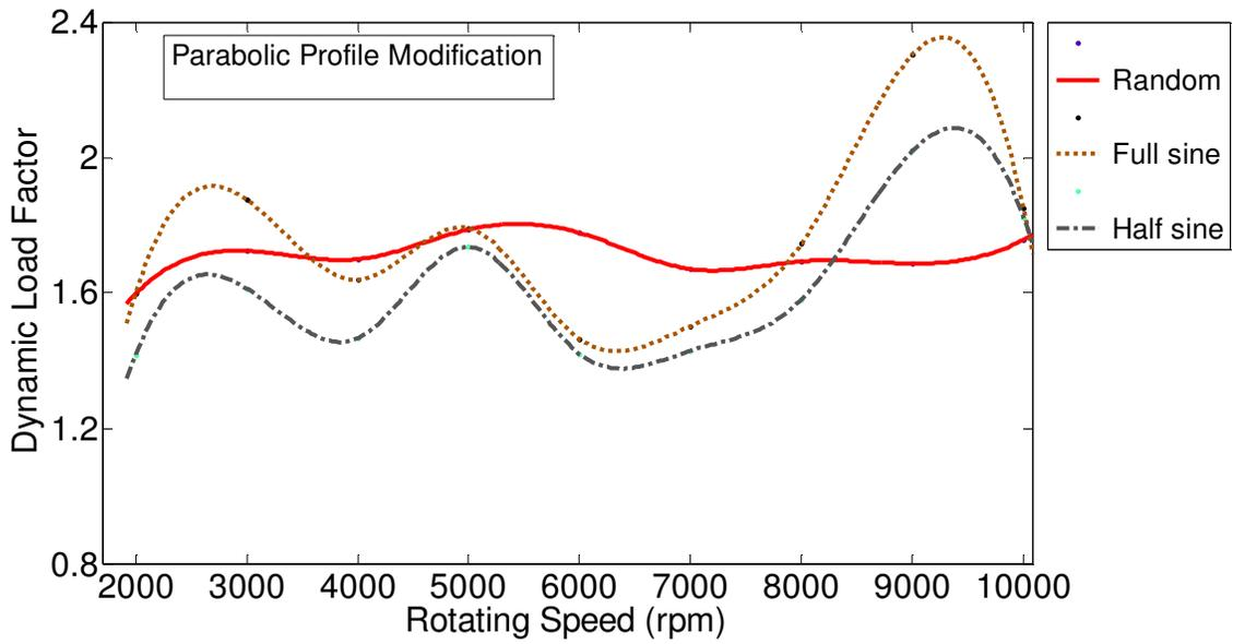
Figure 3.38 Dynamic load factors of sample gears with random, full-sine and half-sine waves of spacing error at 0.0003 in and parabolic profile modification.
