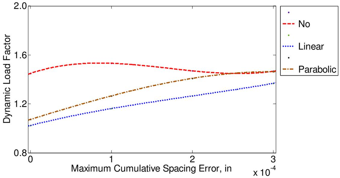
Figure 3.5 Full-sine type of spacing error with no-modification, linear and parabolic profile modifications ( $\Delta=100\%$ ,  $L_n=100\%$ ).
