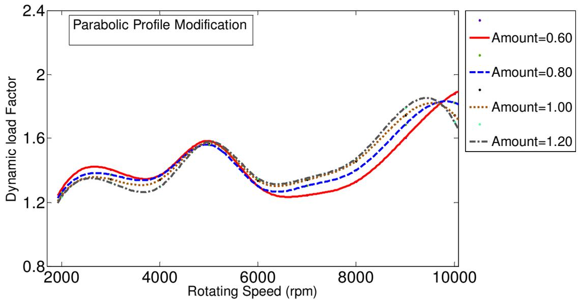
Figure 3.72 Effect of profile modification amount on the gear dynamics, for parabolic tooth profile modification with maximum cumulative half-sine type tooth spacing error of 0.0002 in. The modification amount varies from 0.60 to 1.20, and the length is 100%.
