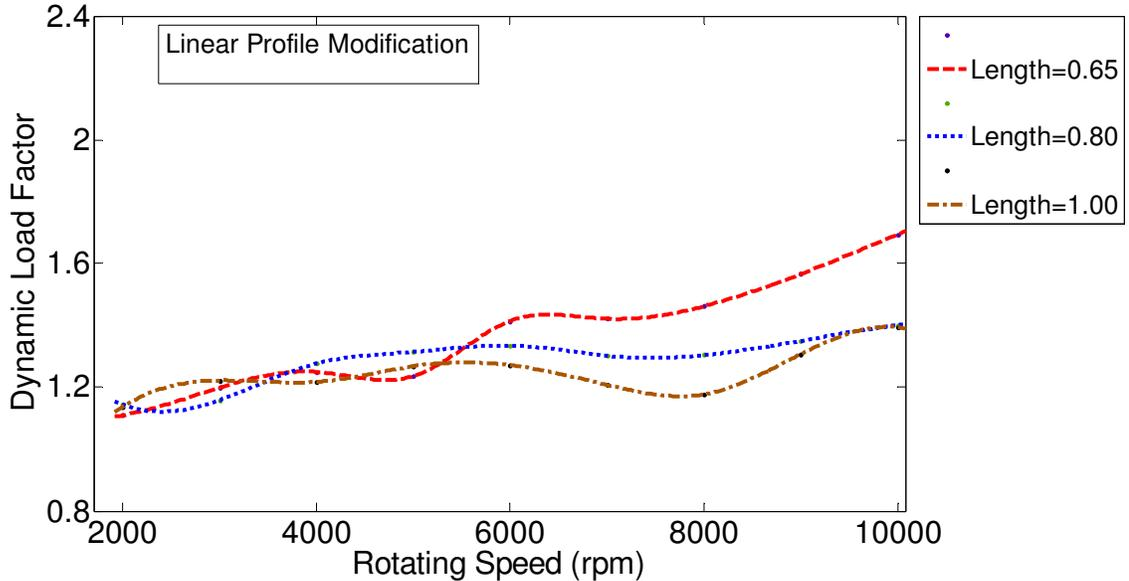
Figure 3.49 Effect of profile modification length on gear dynamic load. Random spacing error with linear profile modification with maximum cumulative tooth spacing error at 0.0001 in ( $\Delta=100\%$ ).
