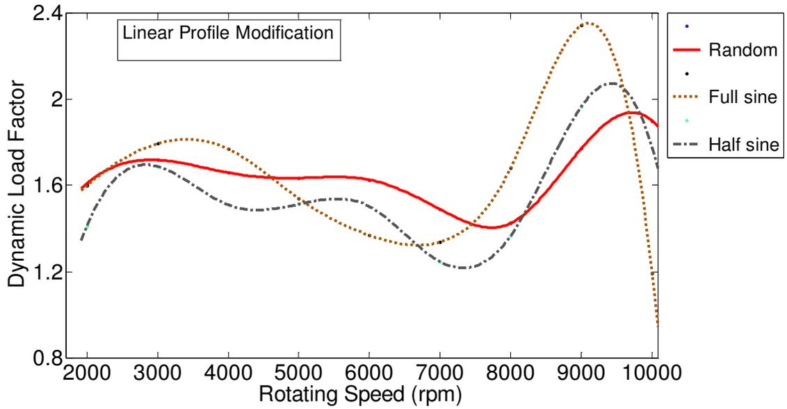
Figure 3.37 Dynamic load factors of sample gears with random, full-sine and half-sine waves of spacing error at 0.0003 in and linear profile modification.
