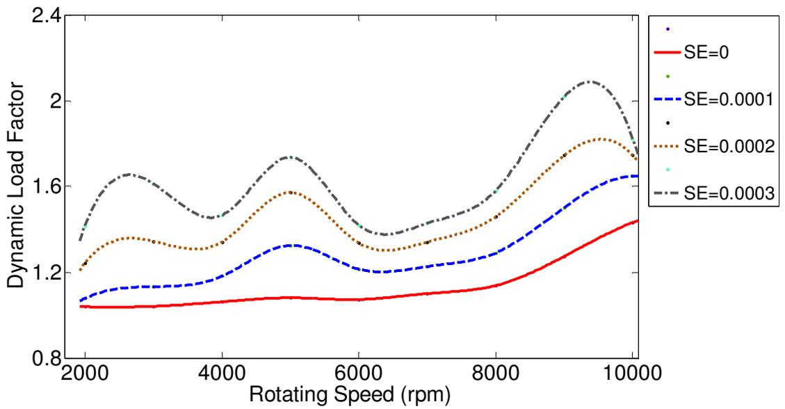
Figure 3.48 Effect of full amount and length of parabolic tooth profile modification with maximum cumulative half-sine type tooth spacing error from 0 to 0.0003 in.
