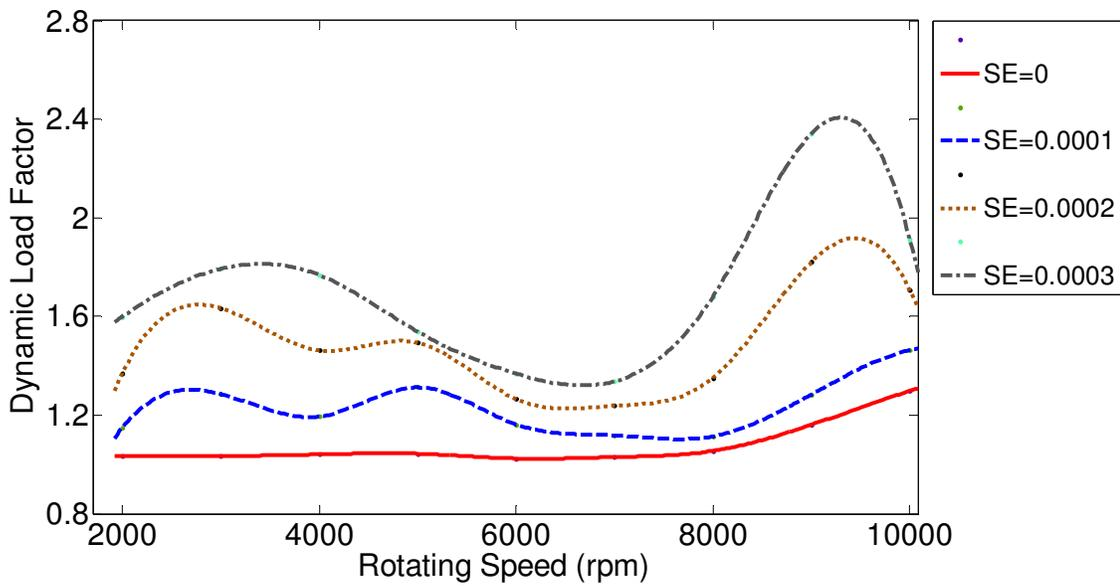
Figure 3.44 Effect of full amount and length of linear tooth profile modification with maximum cumulative full-sine type tooth spacing error from 0 to 0.0003 in.
