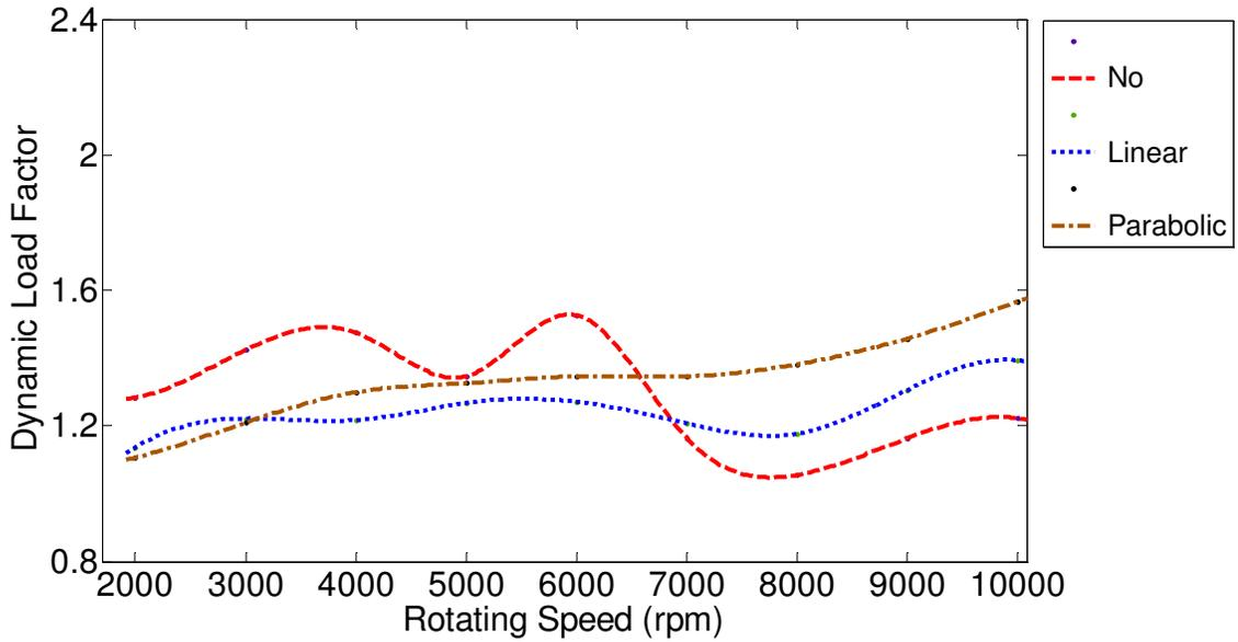
Figure 3.28 Full amount and length of tooth profile modification with maximum cumulative random tooth spacing error of 0.0001 in.
