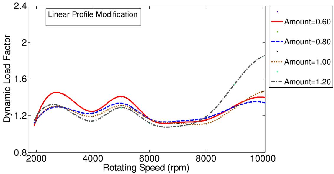
Figure 3.62 Effect of profile modification amount on gear dynamics, for linear tooth profile modification with maximum cumulative full-sine type tooth spacing error of 0.0001 in. The modification amount varies from 0.60 to 1.20, and the length is 100%.
