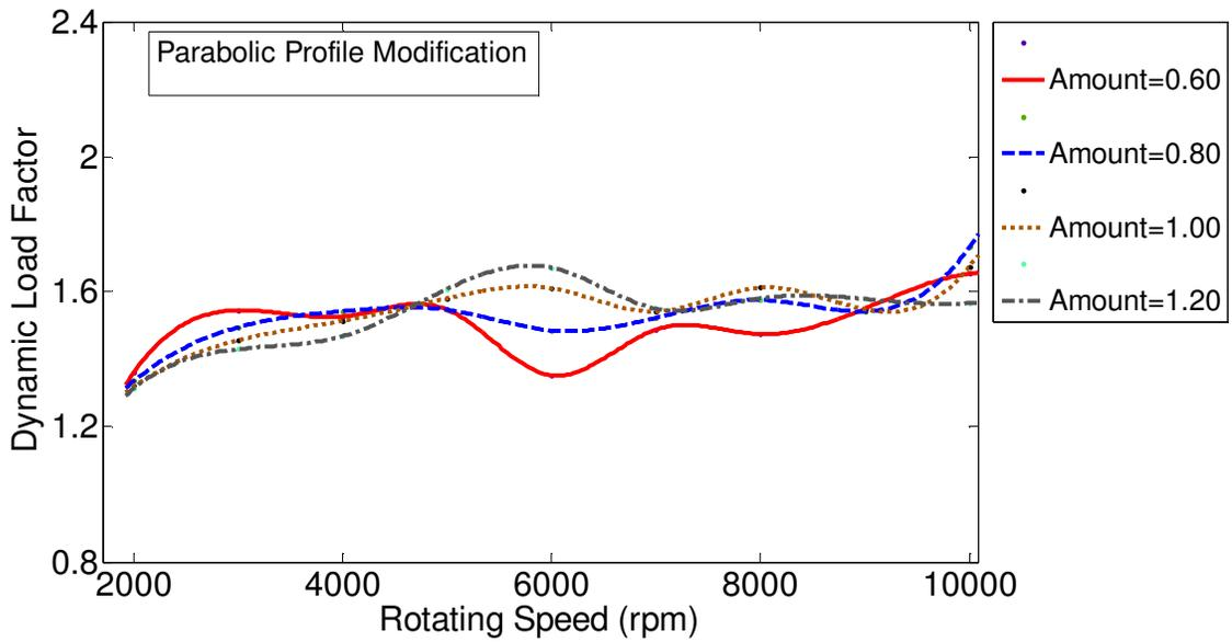
Figure 3.70 Effect of profile modification amount on the gear dynamics, for parabolic tooth profile modification with maximum cumulative random type tooth spacing error of 0.0002 in. The modification amount varies from 0.60 to 1.20, and the length is 100%.
