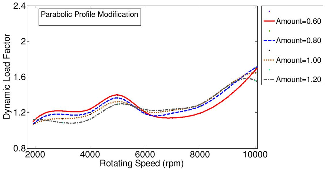
Figure 3.66 Effect of profile modification amount on gear dynamics, for parabolic tooth profile modification with maximum cumulative half-sine type tooth spacing error of 0.0001 in. The modification amount varies from 0.60 to 1.20, and the length is 100%.
