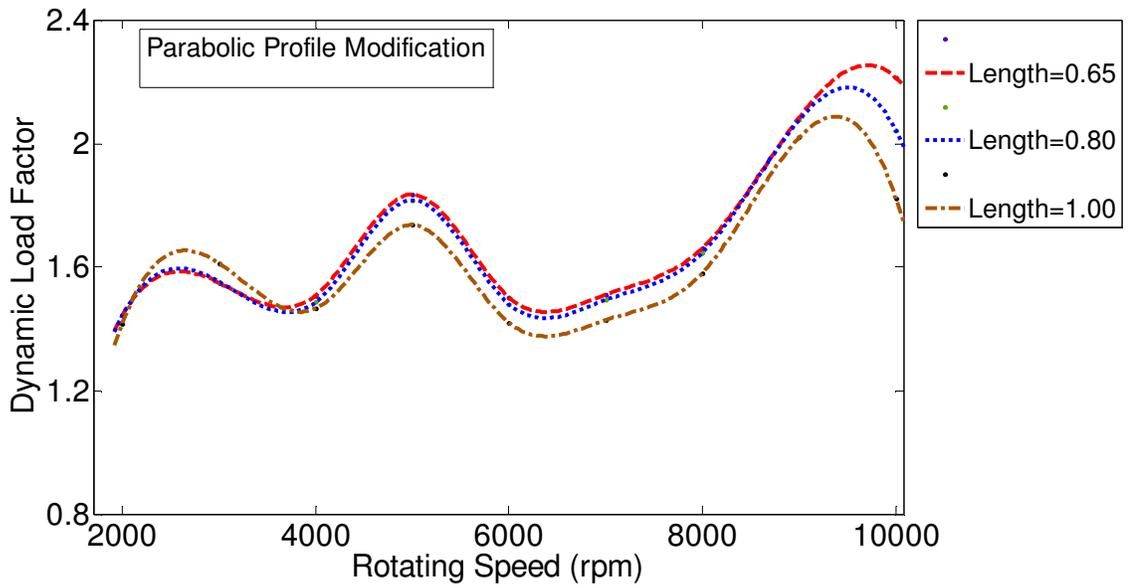
Figure 3.60 Effect of profile modification length on gear dynamic load. Half-sine spacing error with parabolic profile modification, and maximum cumulative tooth spacing error at 0.0003 in ( $\Delta=100\%$ ).
