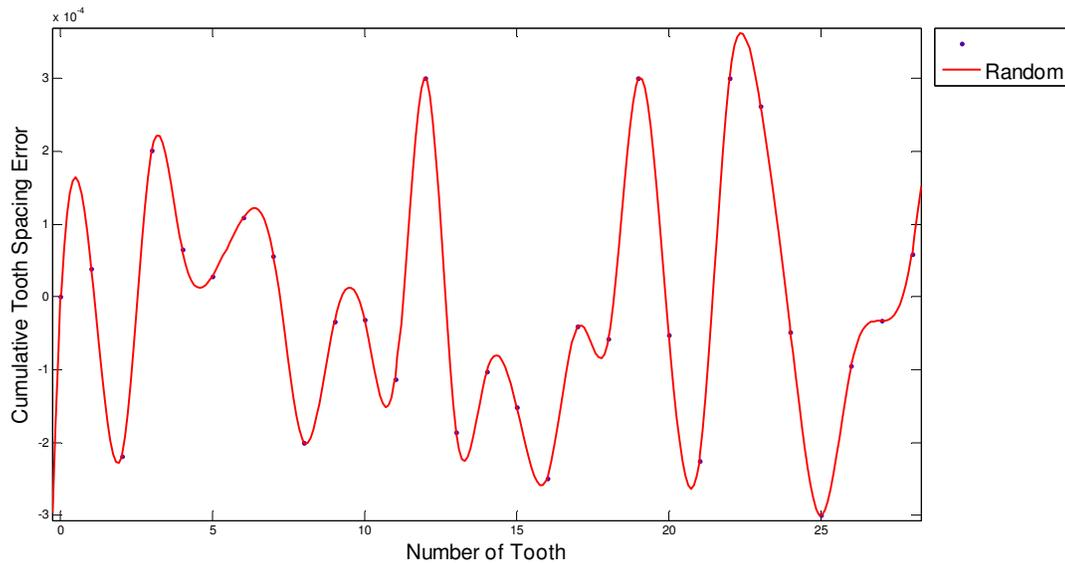
Figure 3.2 Random form cumulative spacing error distribution for a 28-teeth gear. The maximum error value is 0.0003in.
