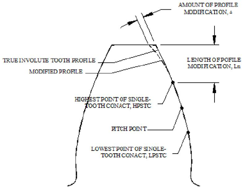
Figure 2.3 Gear tooth with profile modification
