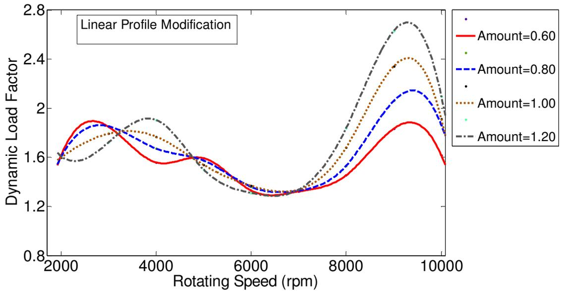
Figure 3.74 Effect of profile modification amount on gear dynamics, for linear tooth profile modification with maximum cumulative full-sine type tooth spacing error of 0.0003 in. The modification amount varies from 0.60 to 1.20, and the length is 100%.
