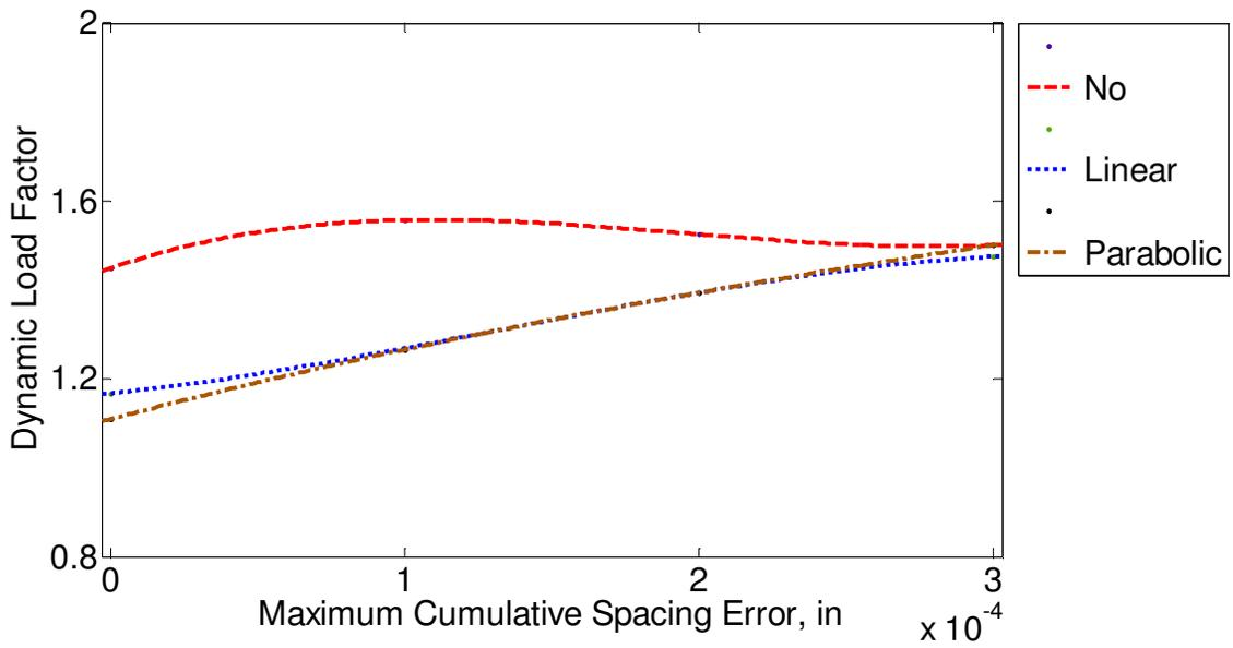
Figure 3.9 Half-sine type of spacing error with no-modification, linear and parabolic profile modifications ( $\Delta=100\%$ ,  $L_n=70\%$ ).
