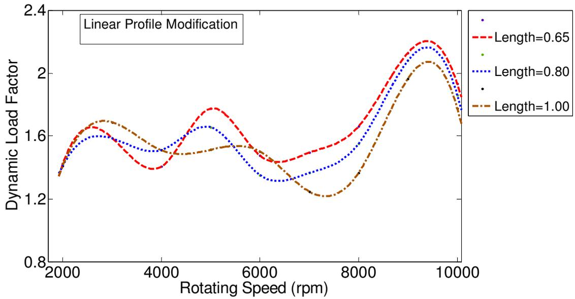
Figure 3.54 Effect of profile modification length on gear dynamic load. Half-sine spacing error with linear profile modification, and maximum cumulative tooth spacing error at 0.0003 in ( $\Delta=100\%$ ).
