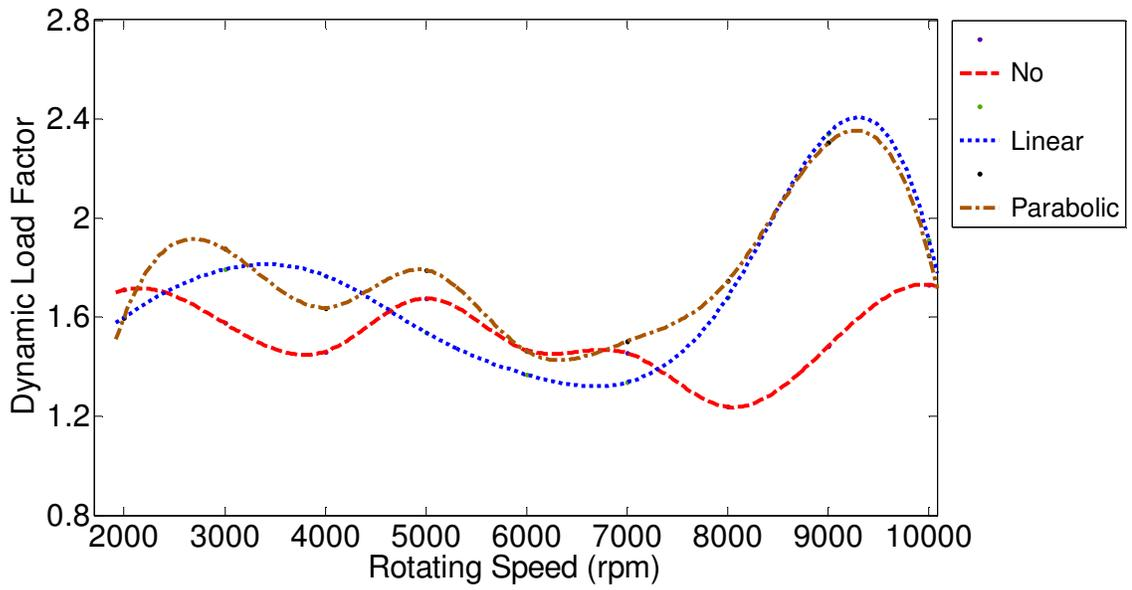
Figure 3.32 Full amount and length of tooth profile modification with maximum cumulative full-sine tooth spacing error of 0.0003 in.
