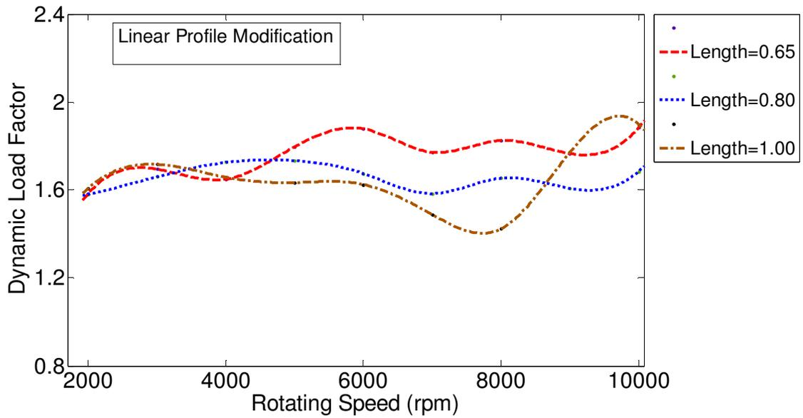
Figure 3.50 Effect of profile modification length on gear dynamic load. Random spacing error with linear profile modification with maximum cumulative tooth spacing error at 0.0003 in ( $\Delta=100\%$ ).
