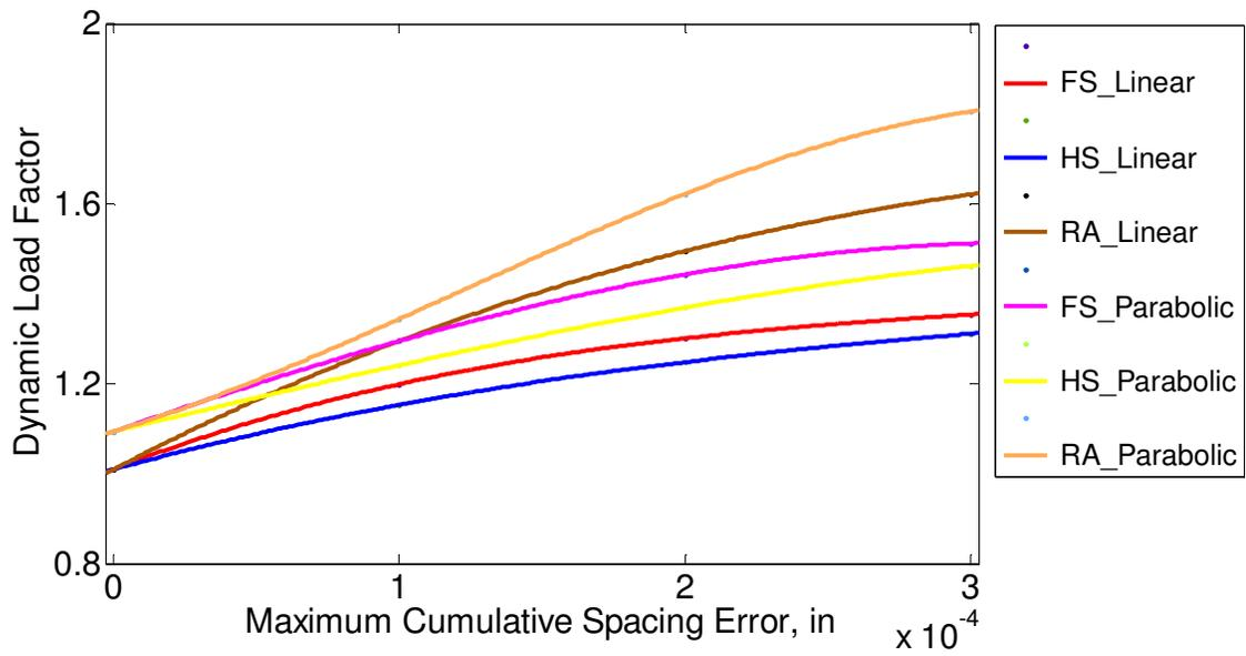
Figure 3.15 Comparison of different type tooth spacing error and profile modifications for ( $\Delta=100\%$ ,  $L_n=85\%$ ).
