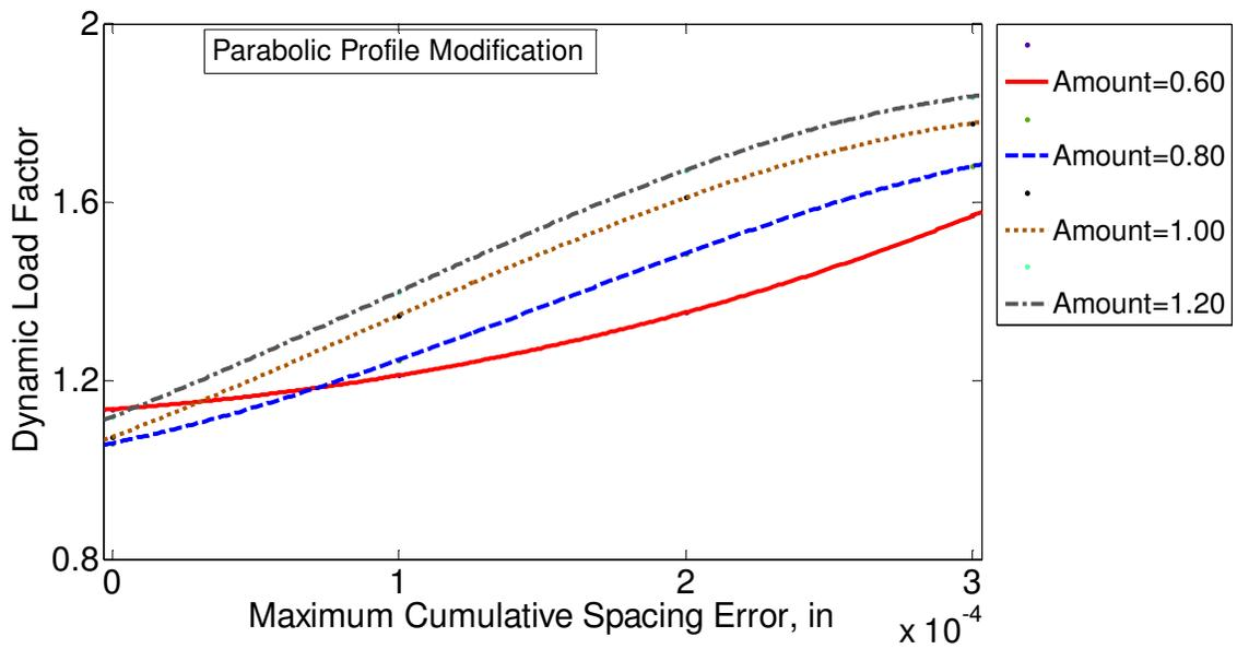
Figure 3.19 Effect of the amount of profile modification on random type of spacing error with parabolic profile modification ( $L_n=100\%$ ).
