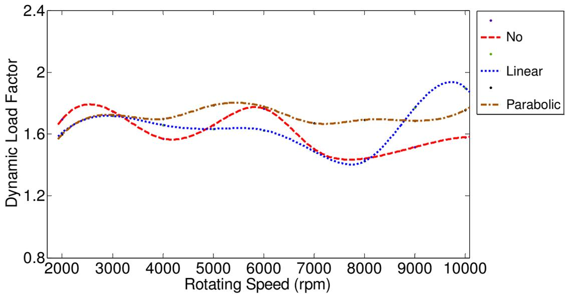
Figure 3.31 Full amount and length of tooth profile modification with maximum cumulative random tooth spacing error of 0.0003 in.
