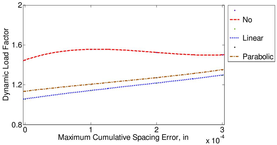
Figure 3.12 Half-sine type of spacing error with no-modification, linear and parabolic profile modifications ( $\Delta=50\%$ ,  $L_n=100\%$ ).
