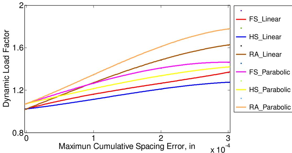
Figure 3.13 Comparison of different type tooth spacing error and profile modifications for ( $\Delta=100\%$ ,  $L_n=100\%$ ).
