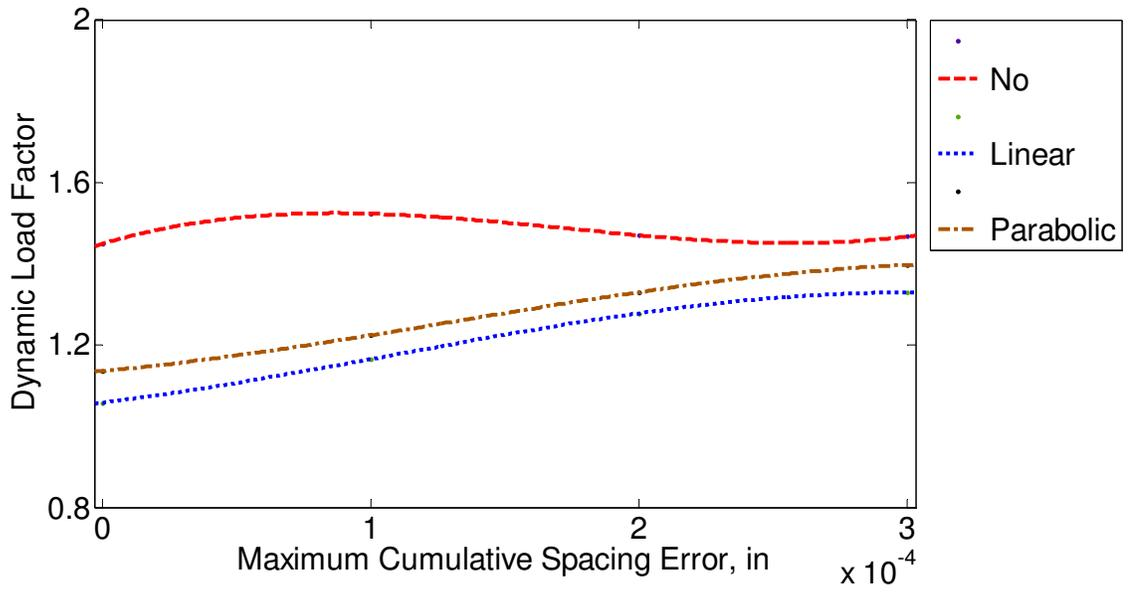
Figure 3.11 Full-sine type of spacing error with no-modification, linear and parabolic profile modifications ( $\Delta=50\%$ ,  $L_n=100\%$ ).
