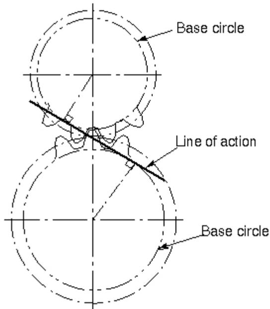
Figure 2.2 Gear line of action
