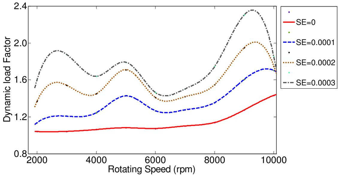
Figure 3.47 Effect of full amount and length of parabolic tooth profile modification with maximum cumulative full-sine type tooth spacing error from 0 to 0.0003 in.
