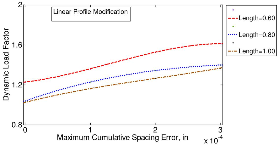
Figure 3.23 Effect of the length of profile modification on full-sine type of spacing error with linear modification ( $\Delta=100\%$ ).
