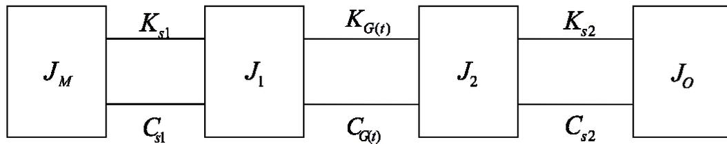
Figure 2.8 Mathematical model of the spur gear system
