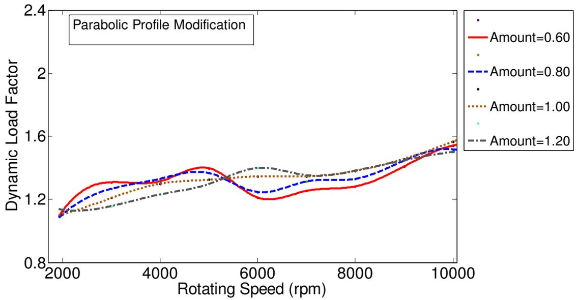
Figure 3.64 Effect of profile modification amount on gear dynamics, for parabolic tooth profile modification with maximum cumulative random type tooth spacing error of 0.0001 in. The modification amount varies from 0.60 to 1.20, and the length is 100%.
