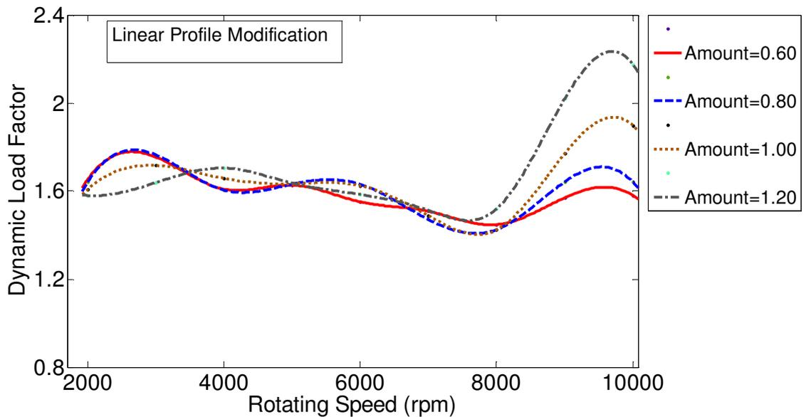
Figure 3.73 Effect of profile modification amount on gear dynamics, for linear tooth profile modification with maximum cumulative random type tooth spacing error of 0.0003 in. The modification varies from 0.60 to 1.20, and the length is 100%.
