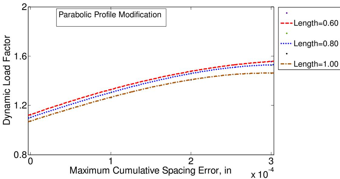
Figure 3.26 Effect of the length of profile modification on full-sine type of spacing error with parabolic modification ( $\Delta=100\%$ ).
