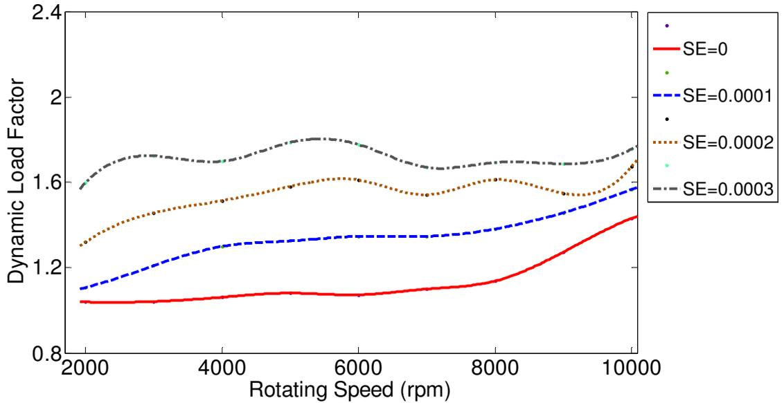
Figure 3.46 Effect of full amount and length of parabolic tooth profile modification with maximum cumulative random type tooth spacing error from 0 to 0.0003 in.
