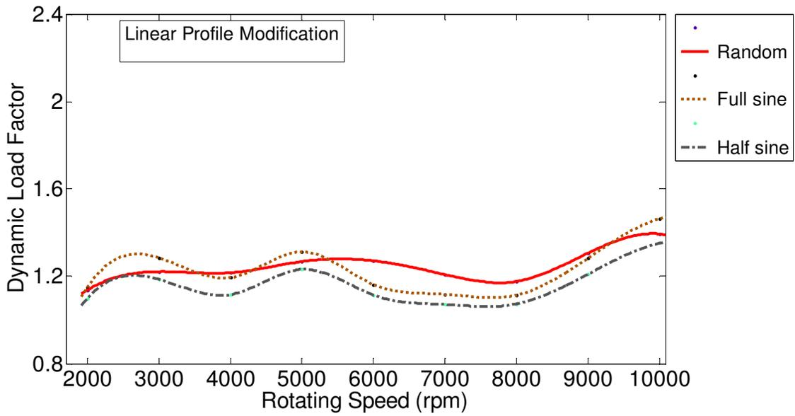
Figure 3.34 Dynamic load factors of sample gears with random, full-sine and half-sine waves of spacing error at 0.0001 in and linear profile modification.
