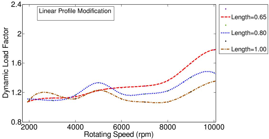
Figure 3.53 Effect of profile modification length on gear dynamic load. Half-sine spacing error with linear profile modification, and maximum cumulative tooth spacing error at 0.0001 in ( $\Delta=100\%$ ).
