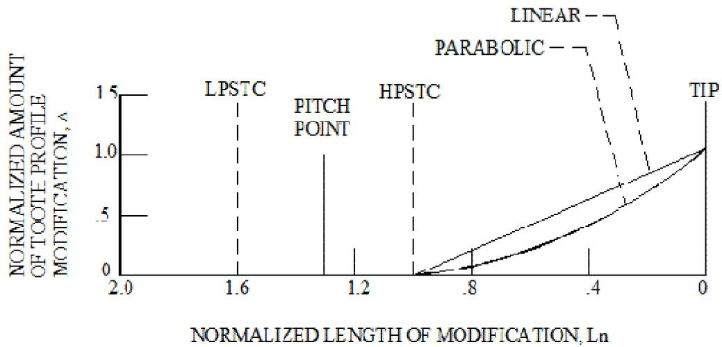
Figure 2.4 Gear tooth with profile modification
