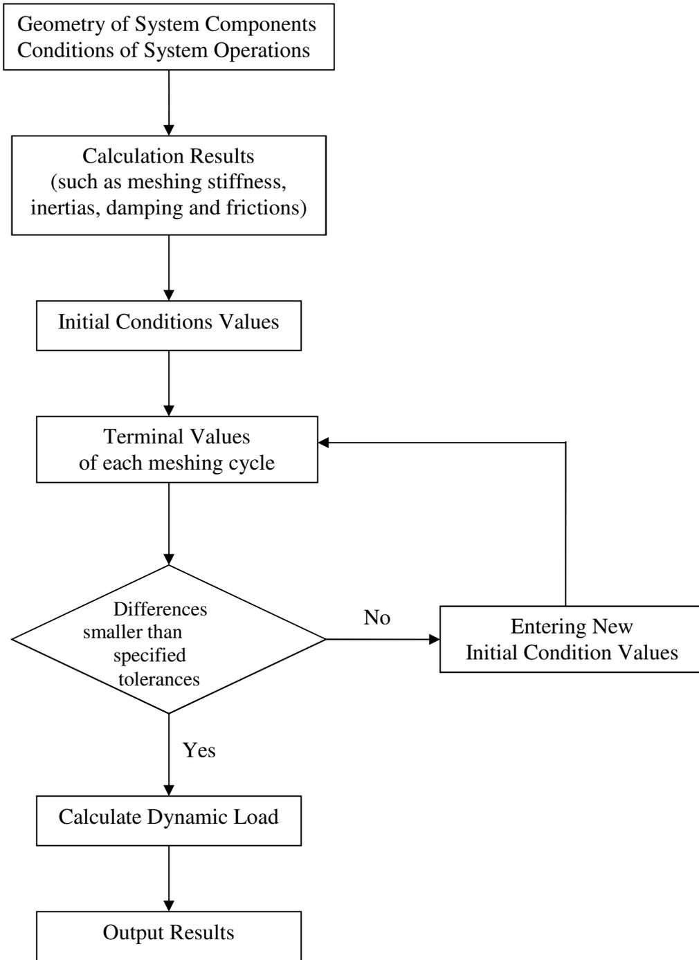
Figure 2.9 Whole procedure of calculating dynamic load
