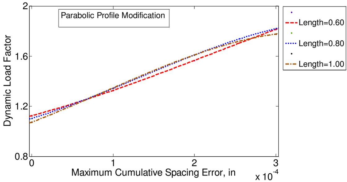
Figure 3.25 Effect of the length of profile modification on random type of spacing error with parabolic modification ( $\Delta=100\%$ ).
