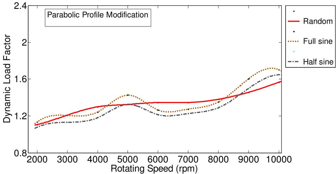
Figure 3.35 Dynamic load factors of sample gears with random, full-sine and half-sine waves of spacing error at 0.0001 in and parabolic profile modification.
