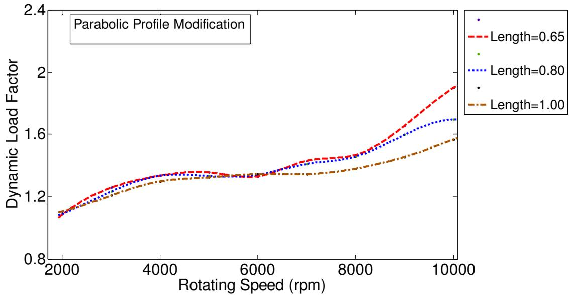
Figure 3.55 Effect of profile modification length on gear dynamic load. Random spacing error with parabolic profile modification, and maximum cumulative tooth spacing error at 0.0001 in ( $\Delta=100\%$ ).
