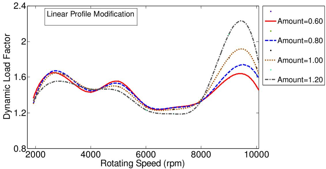
Figure 3.68 Effect of profile modification amount on gear dynamics, for linear tooth profile modification with maximum cumulative full-sine type tooth spacing error of 0.0002 in. The modification amount varies from 0.60 to 1.20, and the length is 100%.
