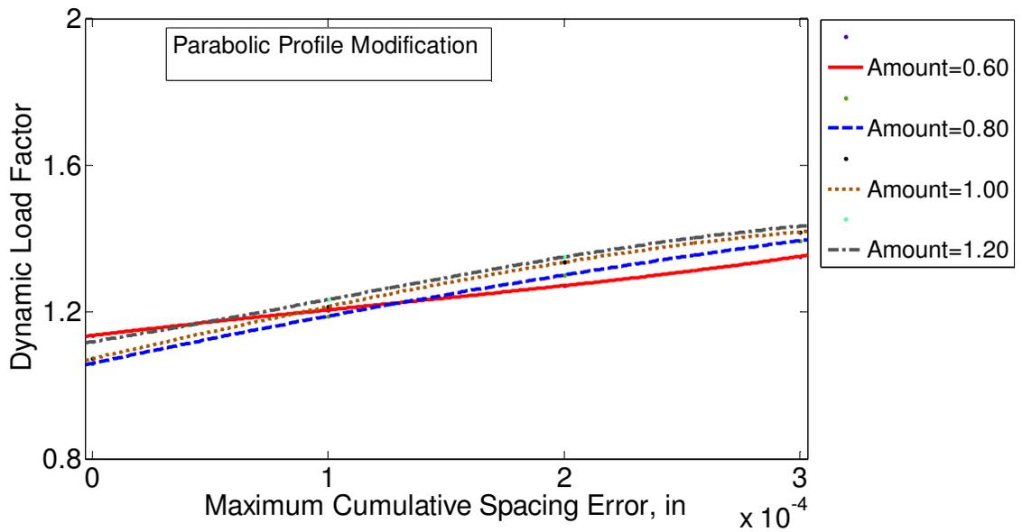
Figure 3.21 Effect of the amount of profile modification on half-sine type of spacing error with parabolic profile modification (Ln=100%).
