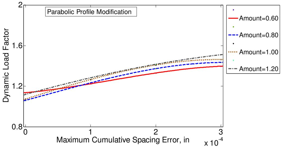
Figure 3.20 Effect the amount of profile modification on full-sine type of spacing error with parabolic profile modification (Ln=100%).
