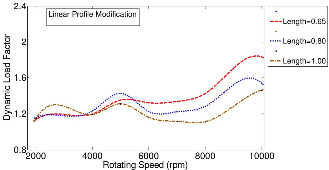
Figure 3.51 Effect of profile modification length on gear dynamic load. Full-sine spacing error with linear profile modification, and maximum cumulative tooth spacing error at 0.0001 in ( $\Delta=100\%$ ).
