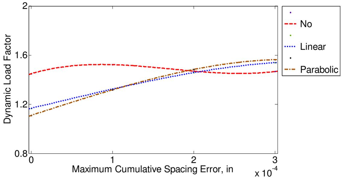
Figure 3.8 Full-sine type of spacing error with no-modification, linear and parabolic profile modifications ( $\Delta=100\%$ ,  $L_n=70\%$ ).
