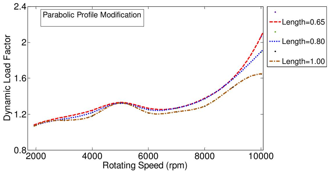
Figure 3.59 Effect of profile modification length on gear dynamic load. Half-sine spacing error with parabolic profile modification, and maximum cumulative tooth spacing error at 0.0001 in ( $\Delta=100\%$ ).
