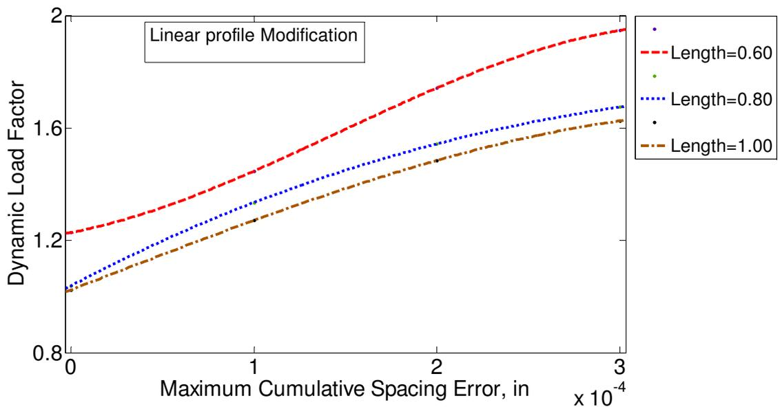
Figure 3.22 Effect of the length of profile modification on random type of spacing error with linear modification ( $\Delta=100\%$ ).
