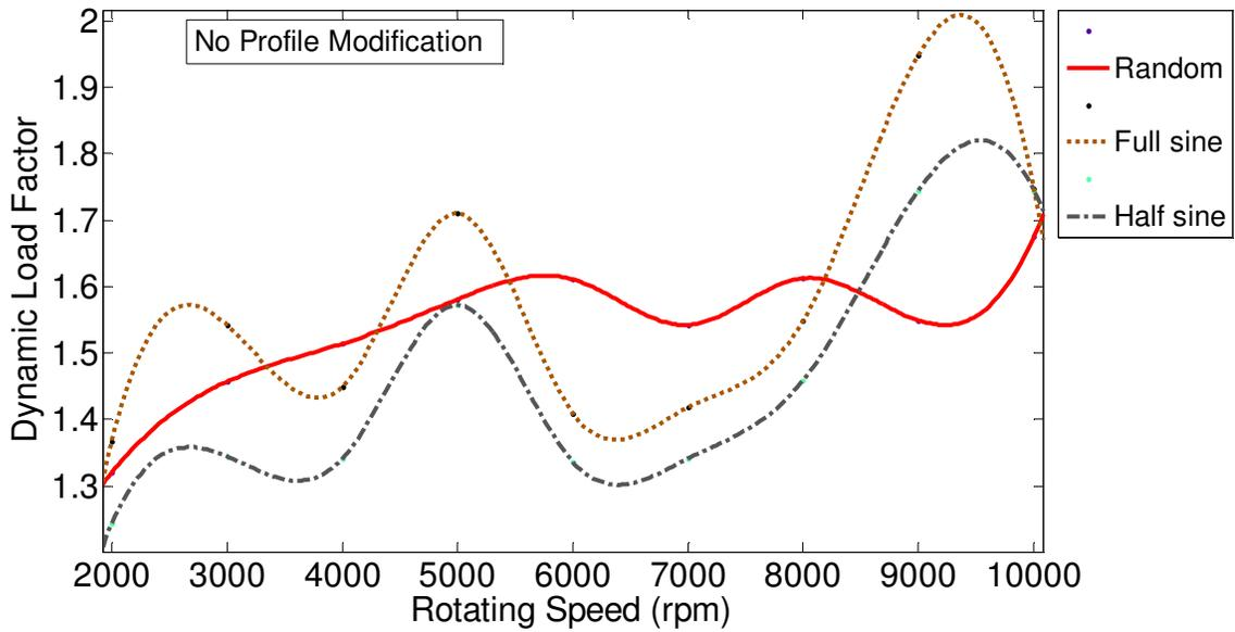
Figure 3.39 Dynamic load factors of sample gears with random, full-sine and half-sine waves of spacing error at 0.0003 in and no profile modification.
