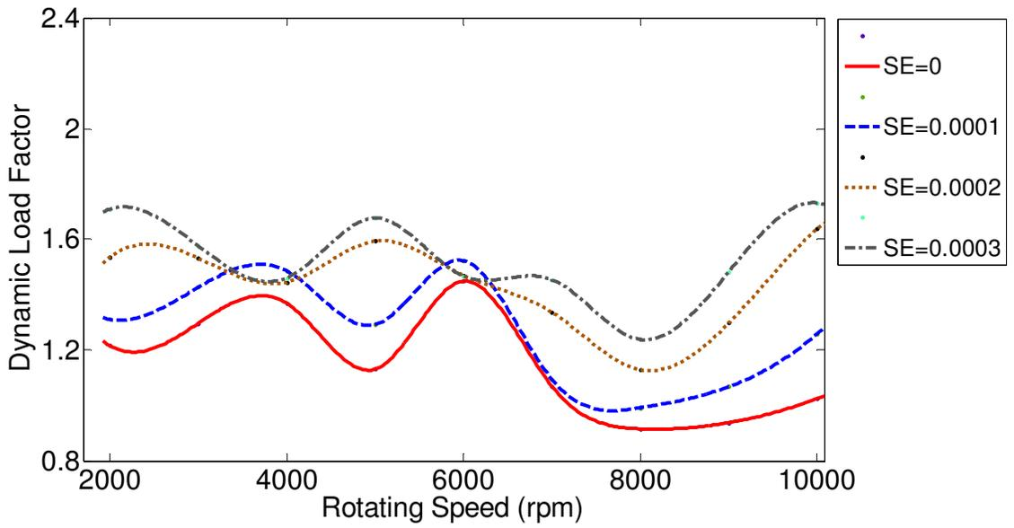
Figure 3.41 Non-modified tooth profile with maximum cumulative full-sine type tooth spacing error from 0 to 0.0003 in.
