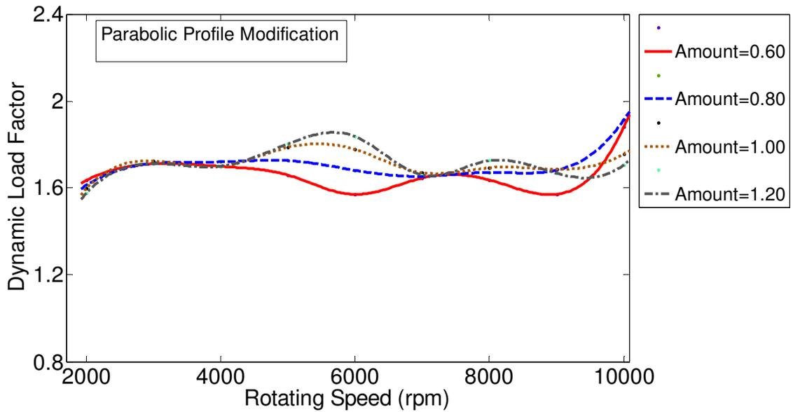
Figure 3.76 Effect of profile modification amount on the gear dynamics, for parabolic tooth profile modification with maximum cumulative random type tooth spacing error of 0.0003 in. The modification amount varies from 0.60 to 1.20, and the length is 100%.
