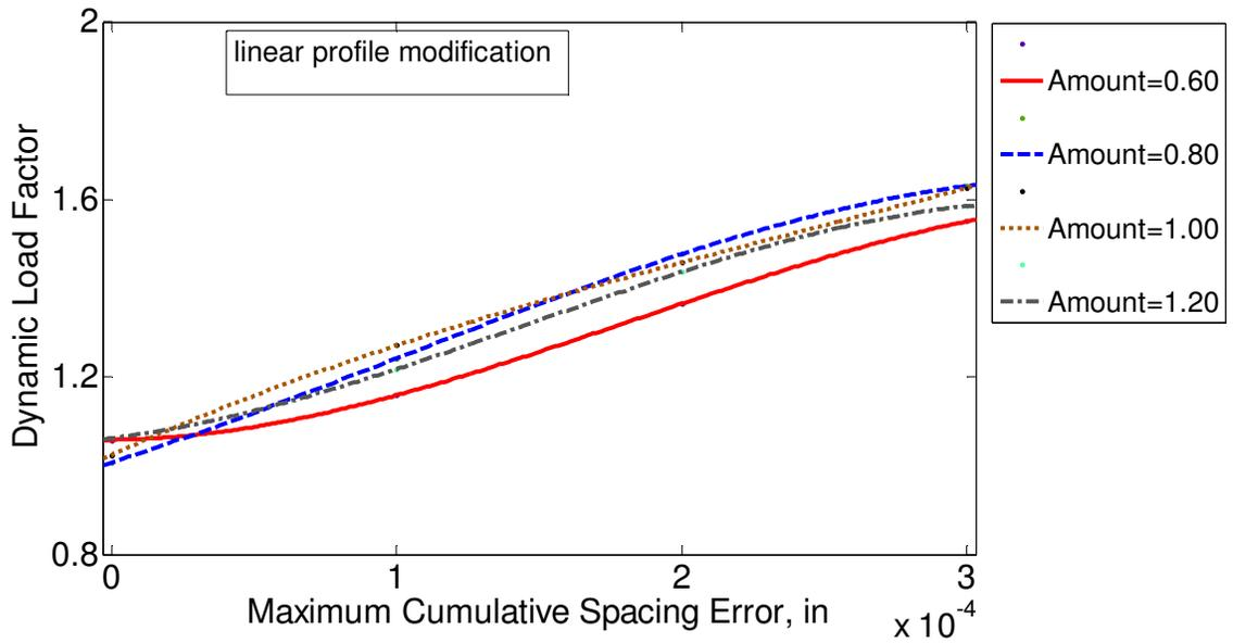
Figure 3.16 Effect of the amount of profile modification on random type of spacing error with linear profile modification (Ln=100%).
