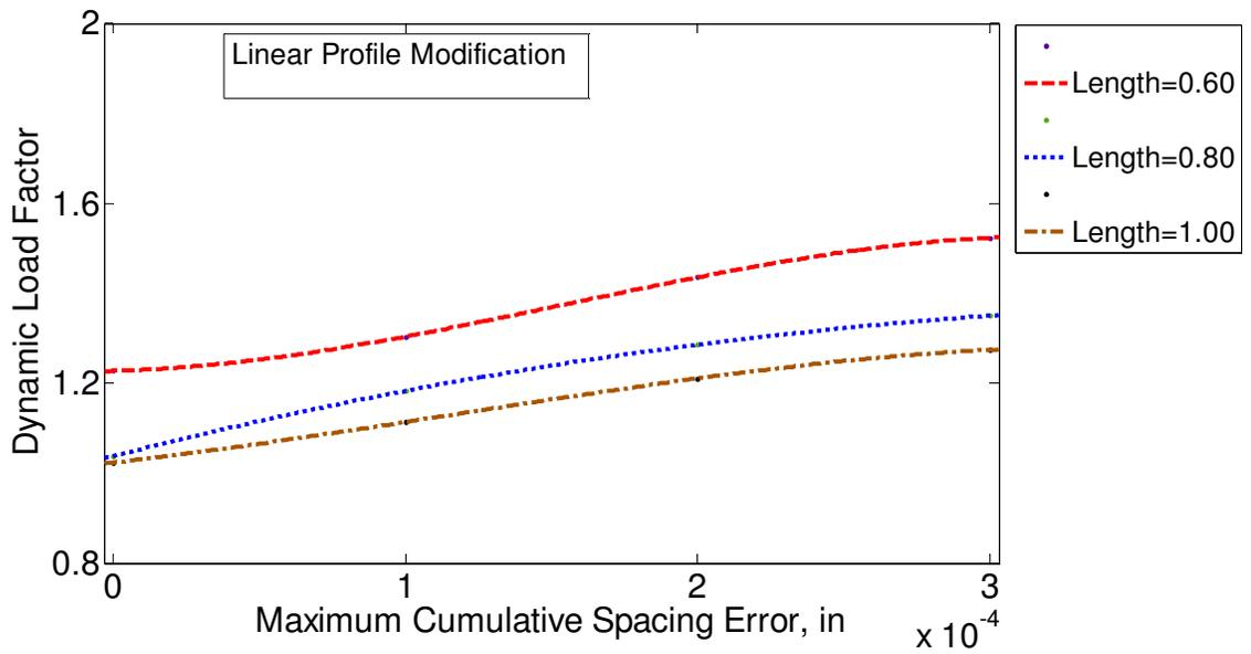
Figure 3.24 Effect of the length of profile modification on half-sine type of spacing error with linear modification ( $\Delta=100\%$ ).
