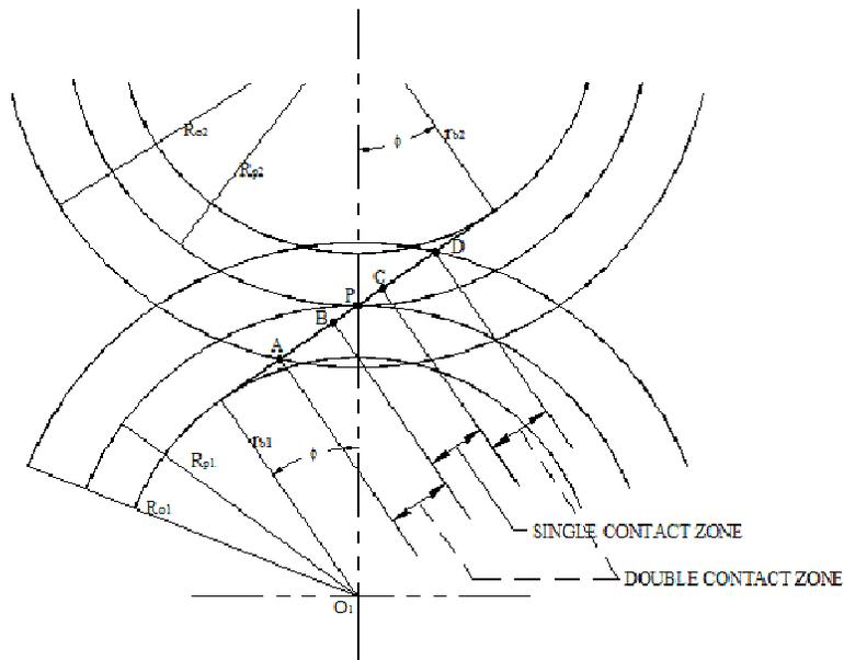
Figure 2.6 - Gear meshing process
