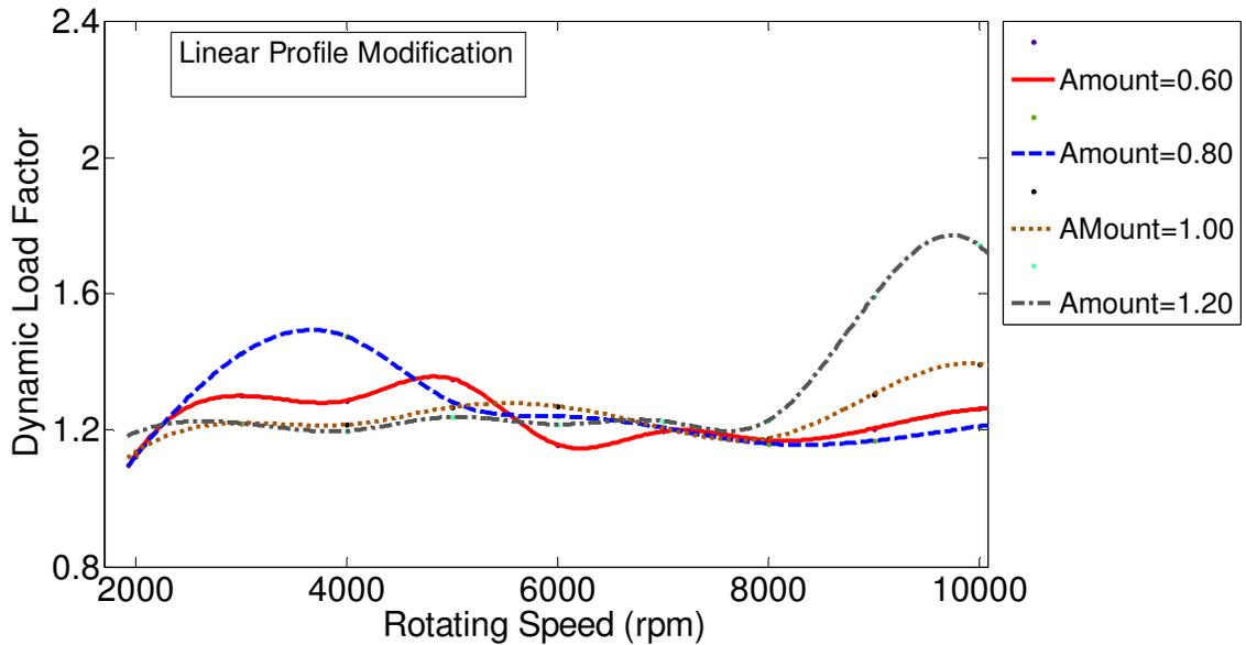
Figure 3.61 Effect of profile modification amount on gear dynamics, for linear tooth profile modification with maximum cumulative random type tooth spacing error of 0.0001 in. The modification amount varies from 0.60 to 1.20, and the length is 100%.
