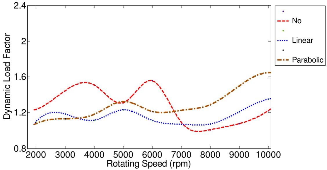
Figure 3.30 Full amount and length of tooth profile modification with maximum cumulative half-sine tooth spacing error of 0.0001 in.
