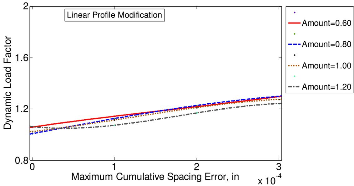
Figure 3.18 Effect of the amount of profile modification on half-sine type of spacing error with linear profile modification ( $L_n=100\%$ ).
