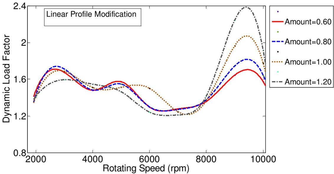
Figure 3.75 Effect of profile modification amount on gear dynamics, for linear tooth profile modification with maximum cumulative half-sine type tooth spacing error of 0.0003 in. The modification amount varies from 0.60 to 1.20, and the length is 100%.
