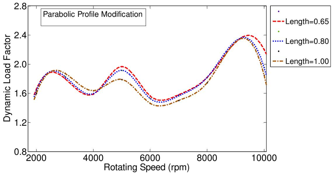
Figure 3.58 Effect of profile modification length on gear dynamic load. Full-sine spacing error with parabolic profile modification, and maximum cumulative tooth spacing error at 0.0003 in ( $\Delta=100\%$ ).
