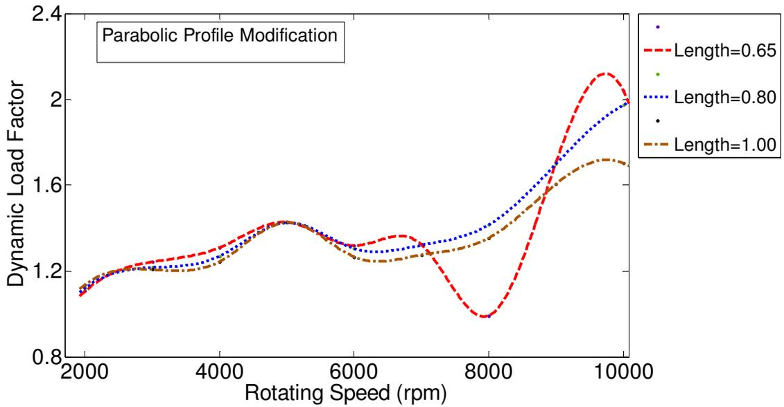
Figure 3.57 Effect of profile modification length on gear dynamic load. Full-sine spacing error with parabolic profile modification, and maximum cumulative tooth spacing error at 0.0001 in ( $\Delta=100\%$ ).
