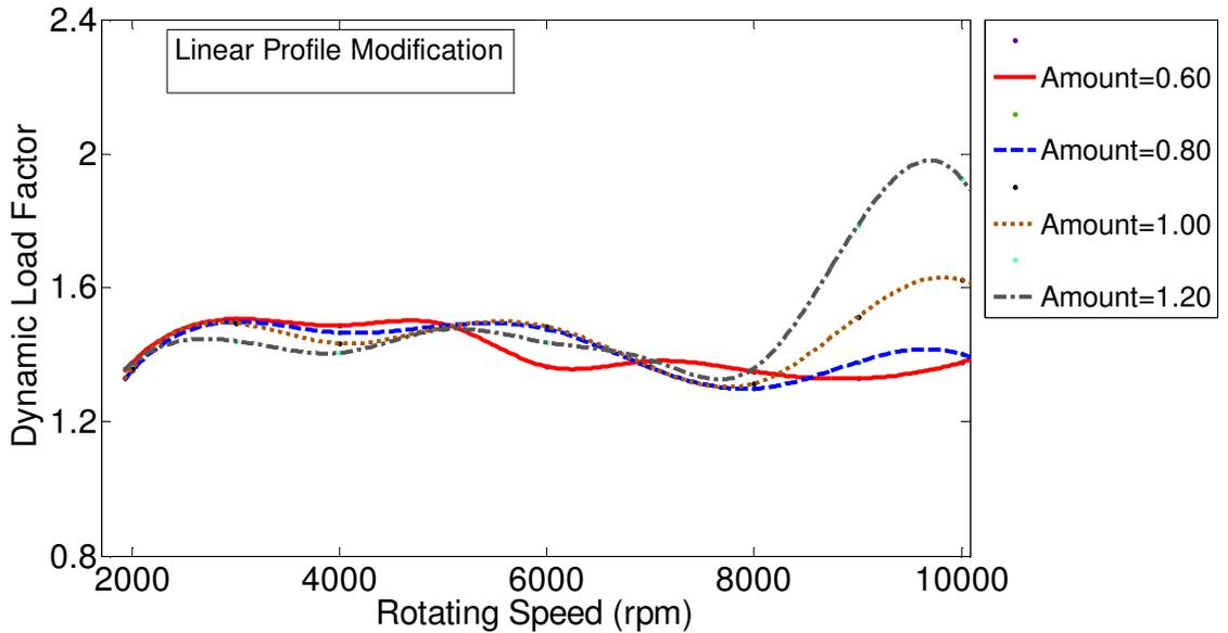
Figure 3.67 Effect of profile modification amount on gear dynamics, for linear tooth profile modification with maximum cumulative random type tooth spacing error of 0.0002 in. The modification amount varies from 0.60 to 1.20, and the length is 100%.
