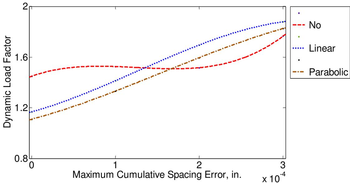
Figure 3.7 Random type of spacing error with no-modification, linear and parabolic modifications ( $\Delta=100\%$ ,  $L_n=70\%$ ).
