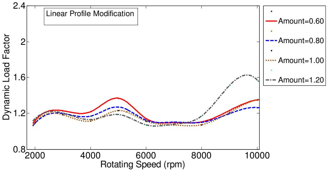
Figure 3.63 Effect of profile modification amount on gear dynamics, for linear tooth profile modification with maximum cumulative half-sine type tooth spacing error of 0.0001 in. The modification amount varies from 0.60 to 1.20, and the length is 100%.
