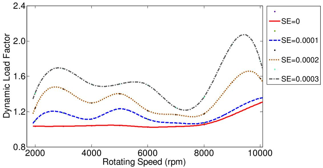
Figure 3.45 Effect of full amount and length of linear tooth profile modification with maximum cumulative half-sine type tooth spacing error from 0 to 0.0003 in.
