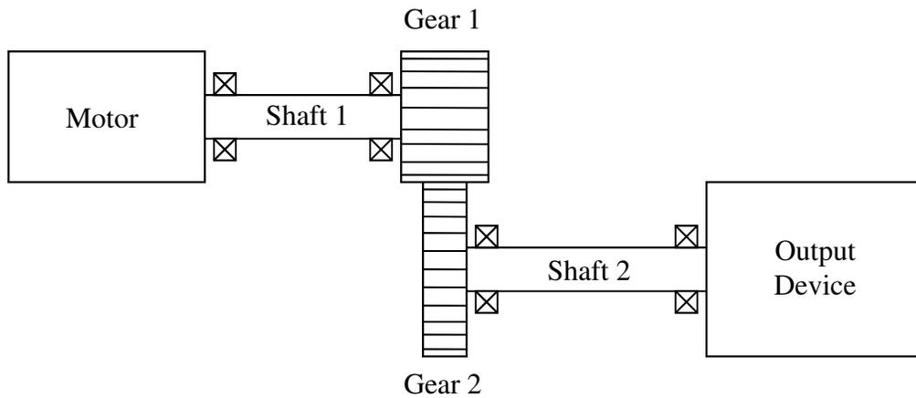
Figure 2.7 Theoretical model of a spur gear system
