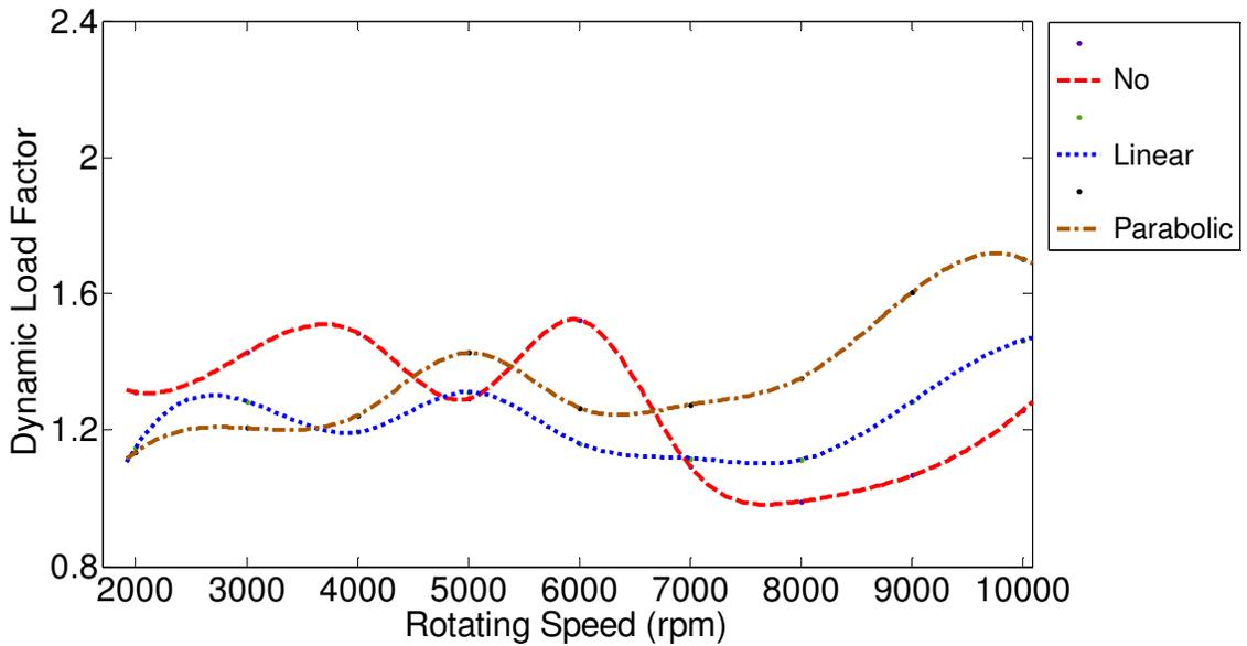
Figure 3.29 Full amount and length of tooth profile modification with maximum cumulative full-sine tooth spacing error of 0.0001 in.
