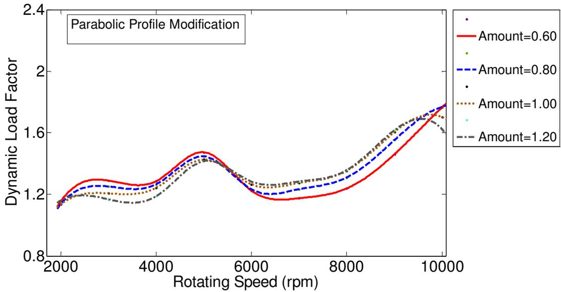
Figure 3.65 Effect of profile modification amount on gear dynamics, for parabolic tooth profile modification with maximum cumulative full-sine type tooth spacing error of 0.0001 in. The modification amount varies from 0.60 to 1.20, and the length is 100%.
