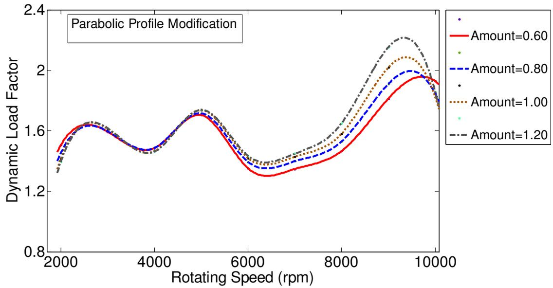
Figure 3.78 Effect of profile modification amount on the gear dynamics, for parabolic tooth profile modification with maximum cumulative half-sine type tooth spacing error of 0.0003 in. The modification amount varies from 0.60 to 1.20, and the length is 100%.
