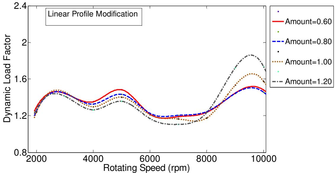
Figure 3.69 Effect of profile modification amount on the gear dynamics, for linear tooth profile modification with maximum cumulative half-sine type tooth spacing error of 0.0002 in. The modification amount varies from 0.60 to 1.20, and the length is 100%.
