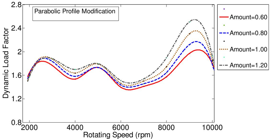
Figure 3.77 Effect of profile modification amount on the gear dynamics, for parabolic tooth profile modification with maximum cumulative full-sine type tooth spacing error of 0.0003 in. The modification amount varies from 0.60 to 1.20, and the length is 100%.
