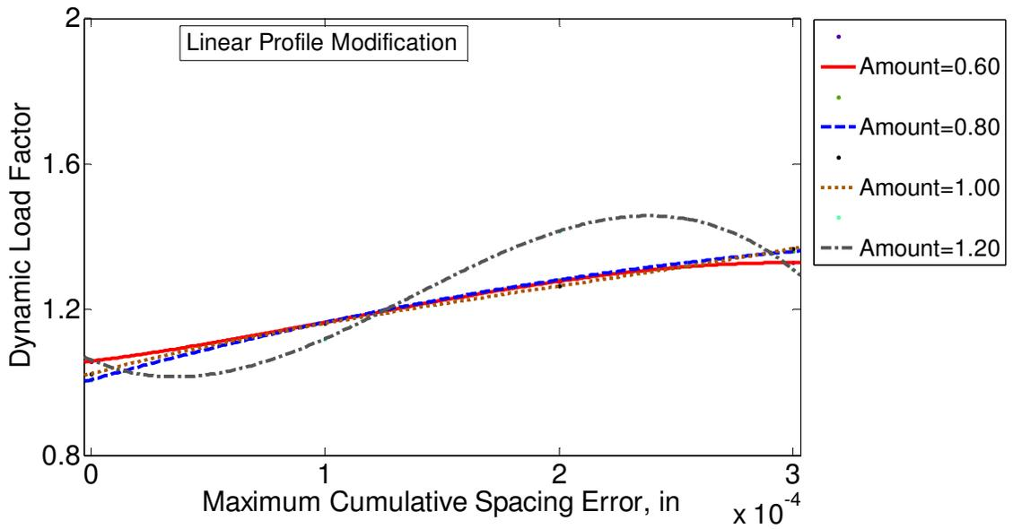
Figure 3.17 Effect of the amount of profile modification on full-sine type of spacing error with linear profile modification (Ln=100%).
