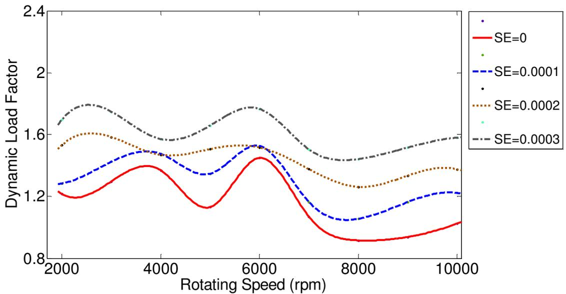
Figure 3.40 Non-modified tooth profile with maximum cumulative random type tooth spacing error from 0 to 0.0003 in.
