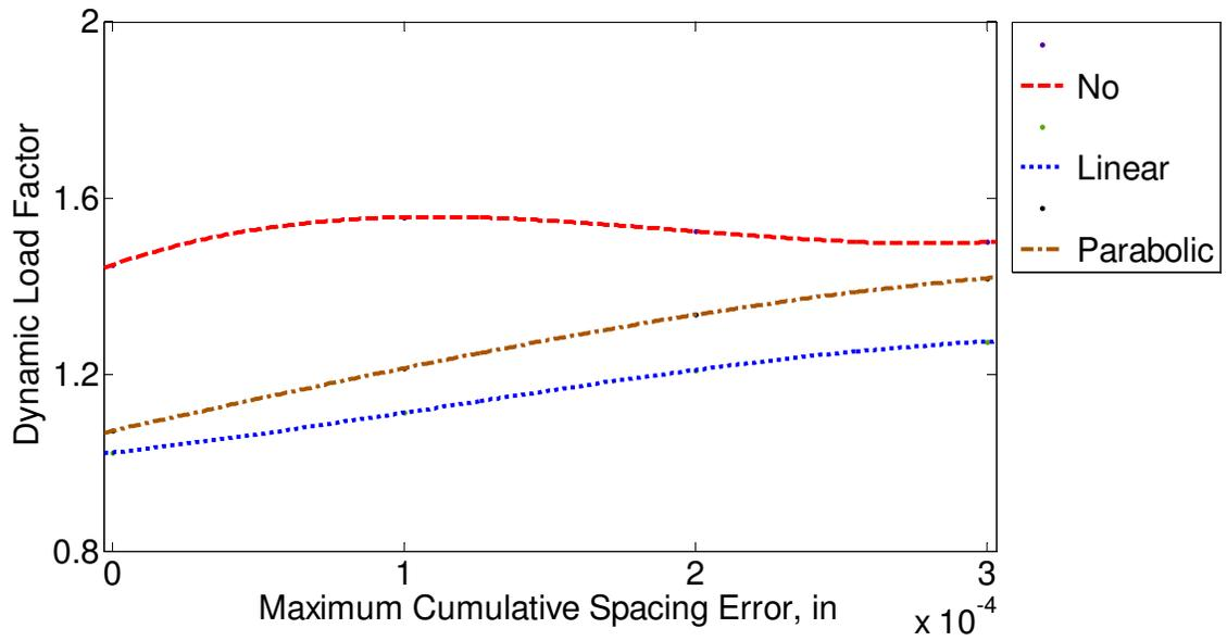
Figure 3.6 Half-sine type of spacing error with no-modification, linear and parabolic profile modifications ( $\Delta=100\%$ ,  $L_n=100\%$ ).
