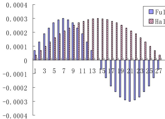
Figure 3.1 Full and Half-sine form cumulative spacing error distribution for a 28-teeth gear. The maximum error value is 0.0003in [3].
