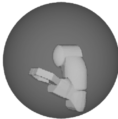
Figure 5.3: The safe region for the robot used in the simulations. The safe region, which is a region assumed to be clear of obstacles that extends in a sphere from the manipulator's shoulder to its elbow, is used to give the robot some freedom of movement for exploration.
