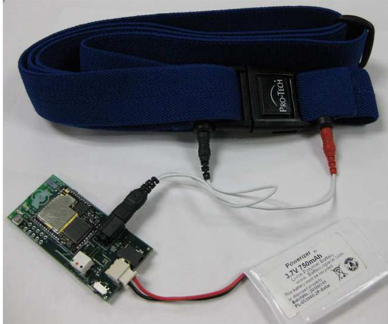
Fig. 3.1: Respiratory Inductive Plethysmograph (RIP) chest band (in blue color) and an uncovered AutoSense sensor board.
