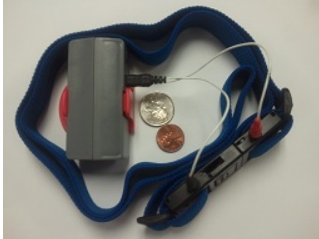
Fig. 3.1: Respiratory Inductive Plethysmograph band (in blue color) is worn around the chest area and the wearable AutoSense sensor unit clips to the belt. A 3-axis Accelerometer, ECG, and Galvanic Skin Response sensors are also included in the same sensor unit. Two coins (a quarter and a penny) are also shown in the picture to indicate the form factor.
