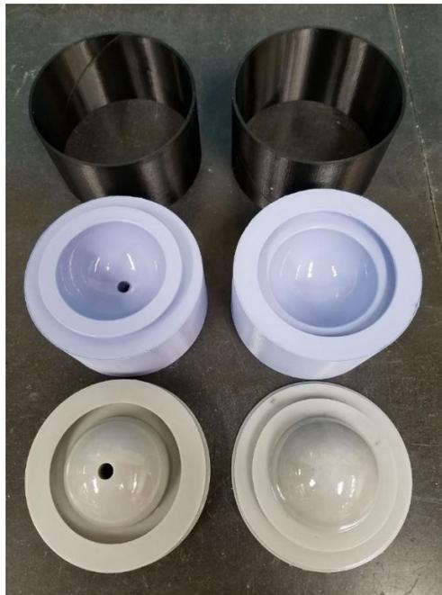
**Figure 1:** Two-piece molds used for casting naphthalene (middle) and mold negatives (top and bottom) used for the construction and curing of the two mold halves [4]. Reprinted with permission.
