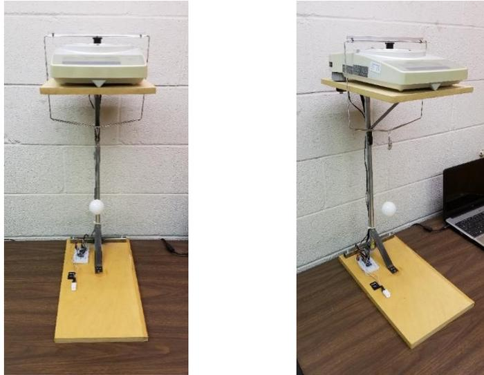
*Figure 2: Scale and weigh-below hook apparatus with suspended specimen for testing [4].
