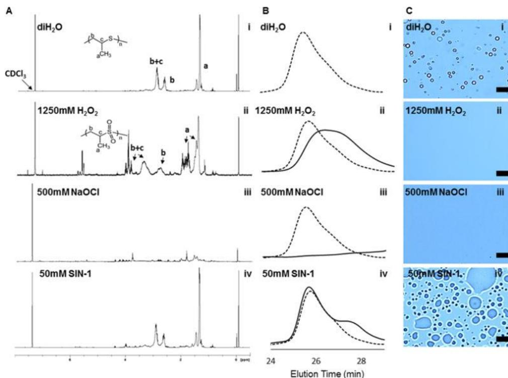
Figure 1: PPS-MS oxidation and subsequent solvation in the presence of hydrogen peroxide and hypochlorous acid (produced by sodium hypochlorite). There is a swelling effect for nitric oxide (produced by SIN-1) but minimal scavenging occurs. In the presence of water, PPS-MS does not dissolve. Adapted from O’Grady et al. and reprinted with permission from American Chemistry Society Biomaterials Science & Engineering [9].
