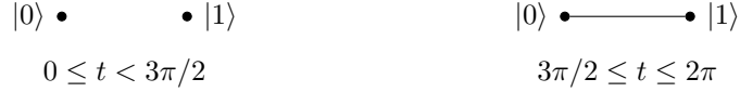
Figure 1.5: A dynamic graph representation of the X gate consists of two graphs and the associated propagation times. This sequence of CTQW executes the logical bit flip operation on the graph state.
